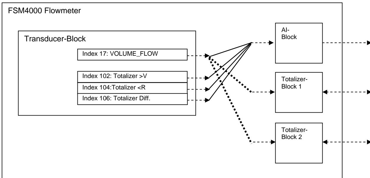
The Totalizer block unit is according to the VOLUME\_FLOW unit, because PA Totalizer blocks are adding up the "VOLUME\_FLOW" value. Example: flow unit: m<sup>3</sup>/h      Totalizer block unit: m<sup>3</sup>.
