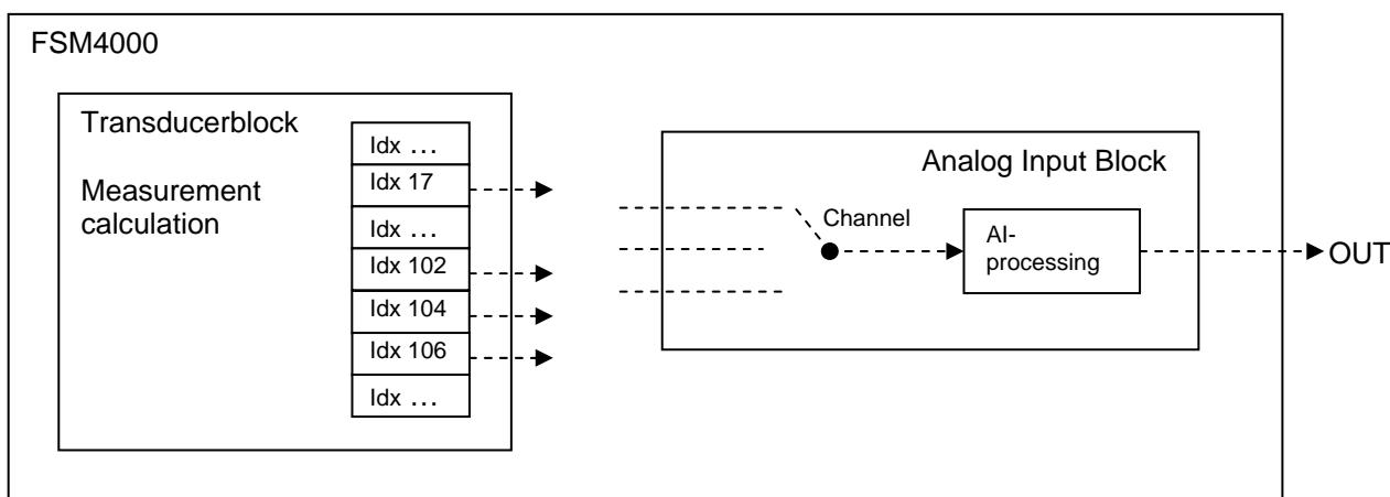
The AI block fulfills certain tasks such as change of scaling, alarm detection, simulation etc. The following section is set out to give you an overview of these tasks.
