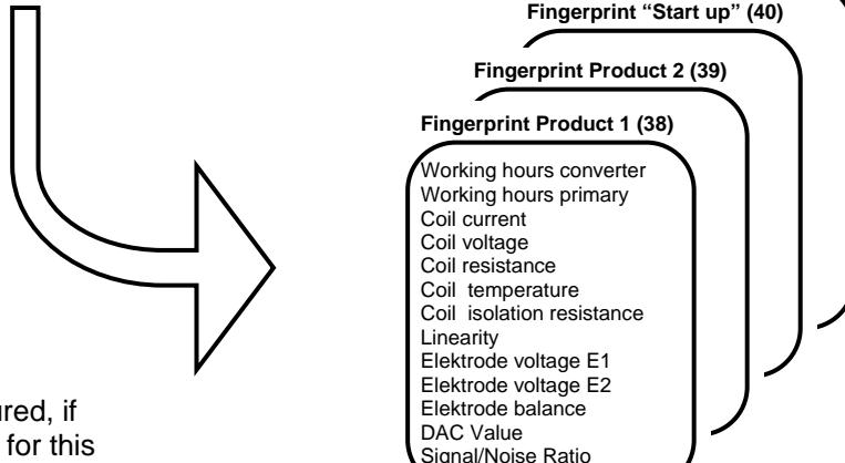
(\*) Some values are only measured, if an error or warning checking for this value is switched on, refer to diagnosis manual.
