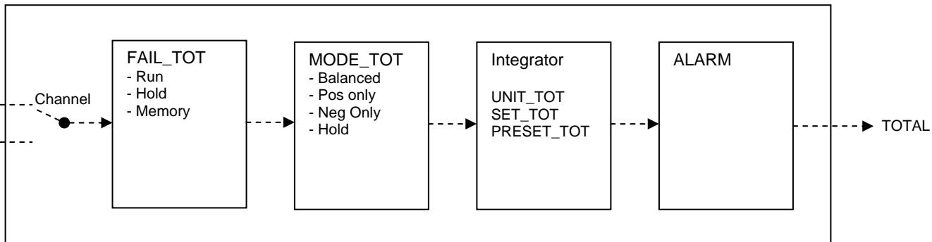
Channel: Measured value from transducer block to be processed can be chosen via channel parameter (index 12). See also 3.5.1
