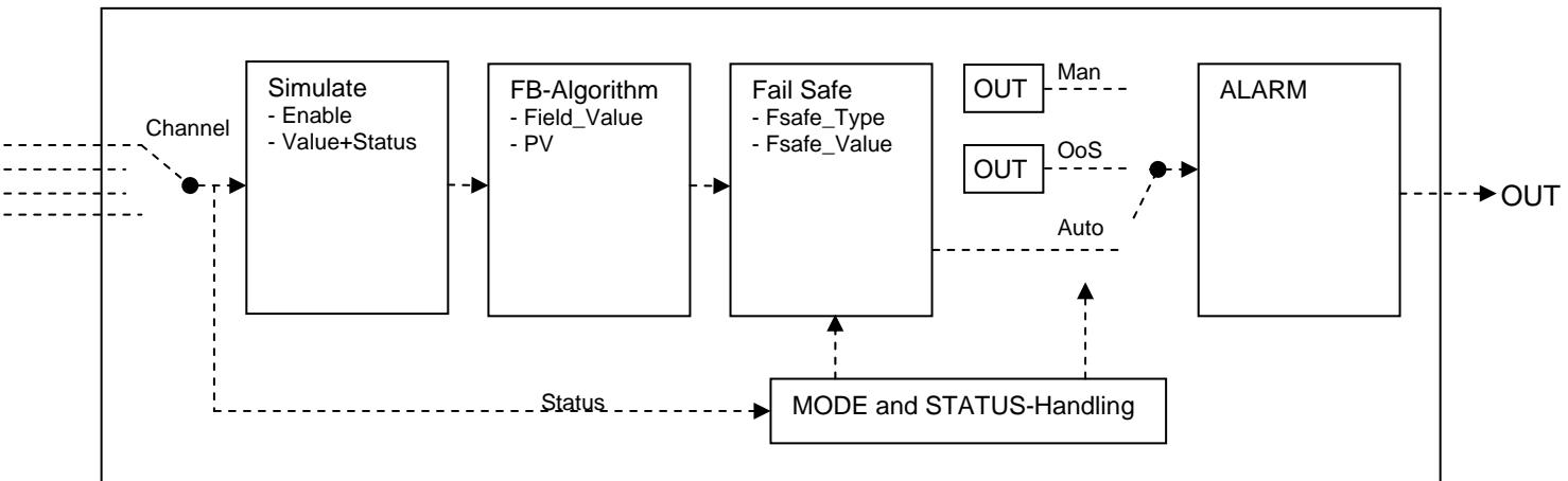
Channel: Please choose the reading to be transferred from the transducer block using the channel parameter (index 14). See also 3.5.1
