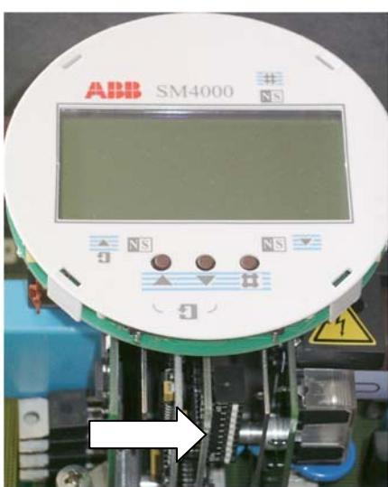
The switch can be seen and set by open converter housing. Take care to security instructions in flowmeter manual before opening the housing. The switch setting is shown on the display in the submenu "data link", menu "Dip Switch". It can also be read by PA communication, Transducerblock relative index 153.
