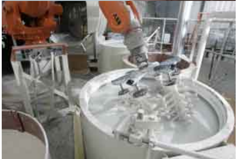
Ceramic shells for making bottles are dipped by an IRB 6600 robot. The uniform dipping makes for higher quality shells.
