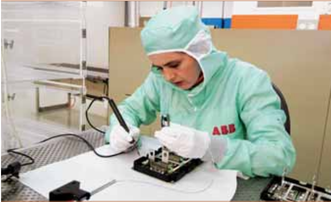
Assembly of a HiPak power semiconductor module
