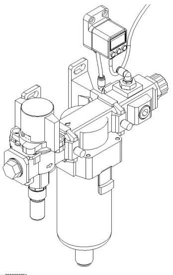
The air supply circuit ends with a Parker Pushlock adapter (suitable for a Parker Pushlock DIN 20 078 A, we recommend a Parker Pushlock 39C82-15-8BK fitting).
