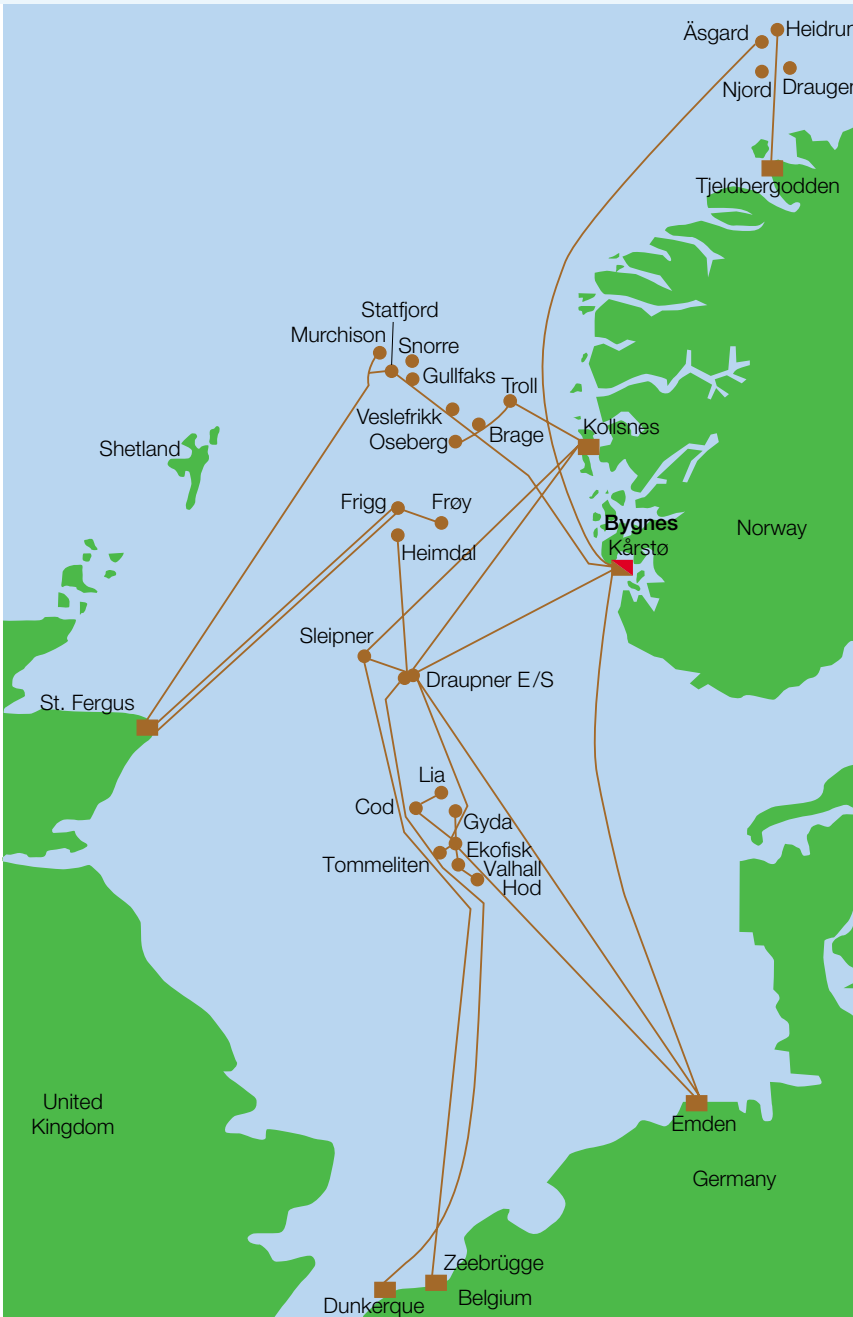
Statoil's Transport Control Center at Bygnes handles 90% of all natural gas from the Norwegian continental shelf and 11% of all natural gas deliveries for Europe. The total length of the Norwegian gas network is 6,500 km. Gas exports are estimated to grow to 65 billion cubic meters in 2000.
