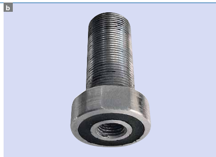
10 An anti-vibration device a b was placed on the RTD sensor c to reduce RTD failures.
