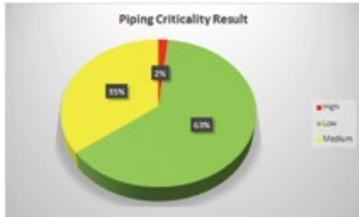
Figure 4. Piping criticality results for typical gas plant.
