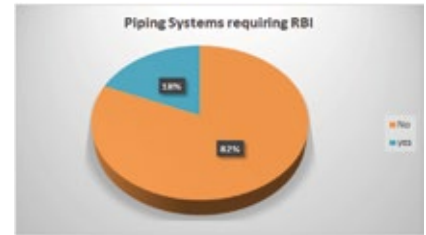
Figure 6. RBI requirement for piping systems.
