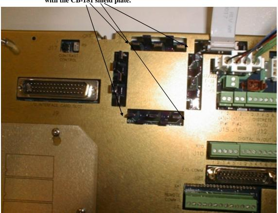
Locations where the heat sink could come into contact with the CB-181 shield plate.
