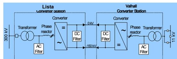
Figure 2. Single Line Diagram of PFS with HVDC.
