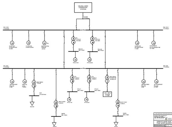
Figure 4. Single line diagram of the AC system on Valhall fed by Power From Shore.
