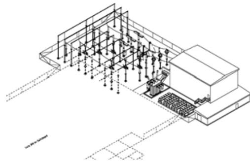
Figure 8. HVDC converter station at Lista
