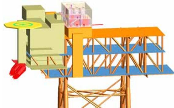
Figure 6. The new Valhall, Production and Hotel platform with the HVDC module on top.
