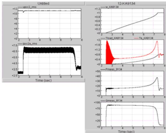
Figure 5. Illustration of DOL motor start
