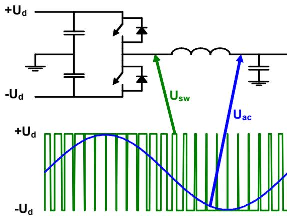
Figure 3. Principle of pulse width modulation, PWM.
