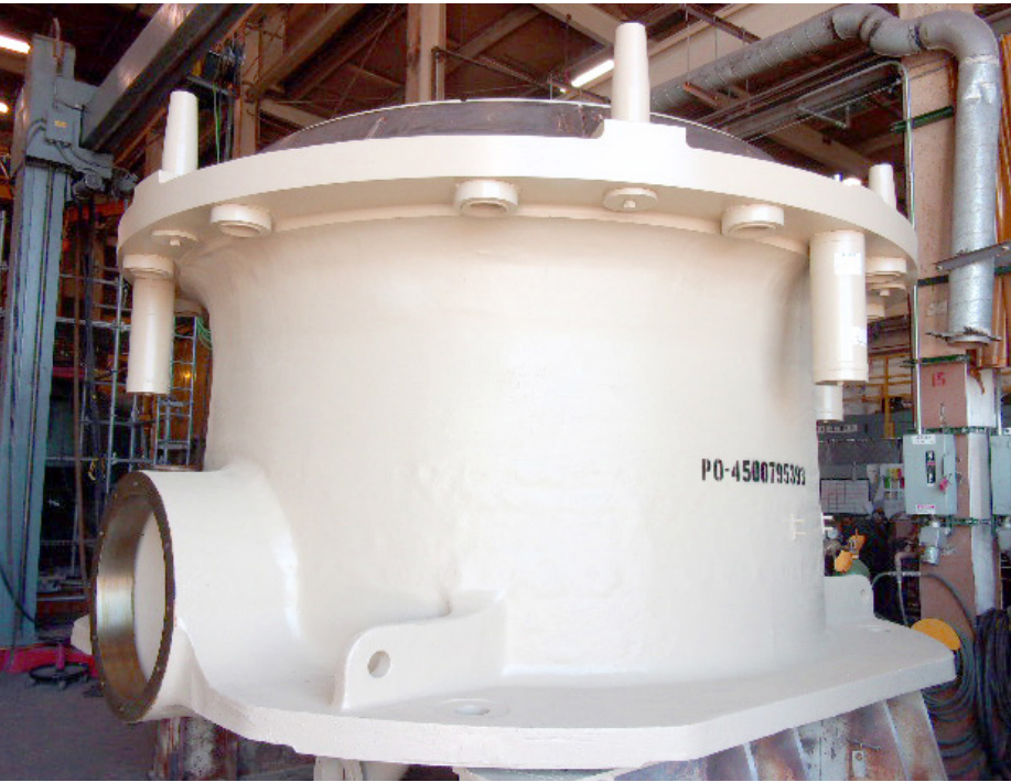
— Rebuilt Crusher Main Frame
