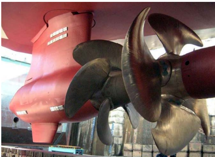
Figure 3-9 The contra-rotating Azipod solution is made together with a traditional shaft line
