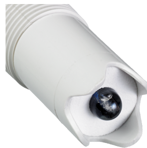
Figure 6 Low temperature (LT) glass with notched body
