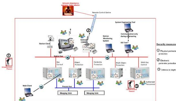
Figure 3: A typical substation automation setup with security mechanisms
