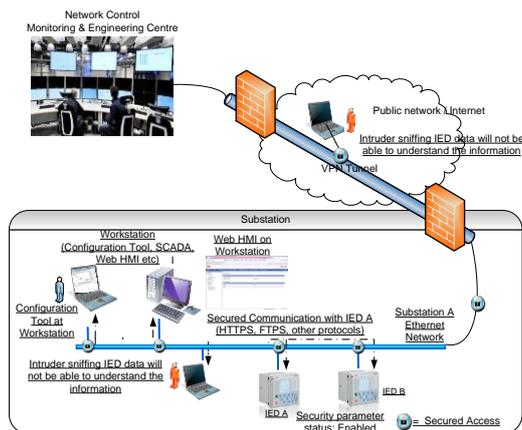
Figure 4: Secure communication through Public Network
