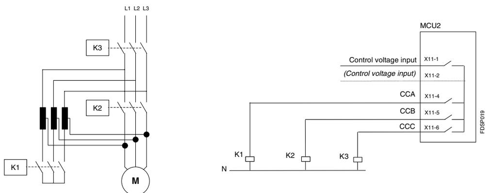
All protection functions are supported by this starter type during normal "Running" situation. For motor starting additional set of protection functions are disabled for the time *Autotrafo start time* parameter defines. For more information see chapter 'Protection functions disabled'.
