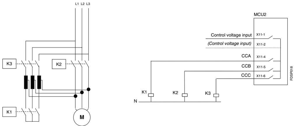
**Picture 33.** Control circuit for autotransformer starter, example 2.
