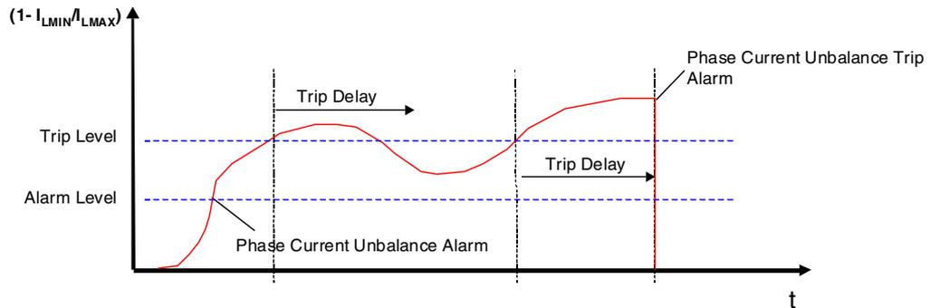
$(1 - I_{Lmin}/I_{Lmax})$  is compared against the unbalance *Alarm level*. When  $(1 - I_{Lmin}/I_{Lmax})$  exceeds above the unbalance *Alarm level*, an “Phase Current Unbalance alarm” alarm is issued.
