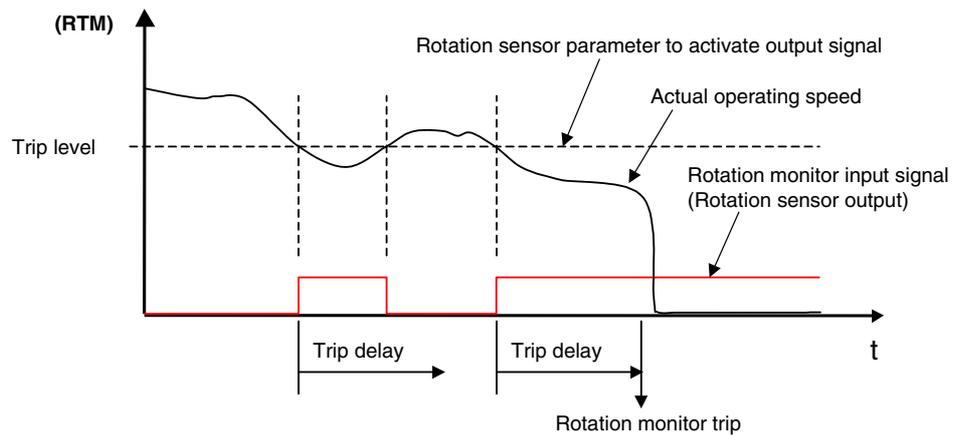
The MCU compares the signal from rotation monitor input to *Trip delay* parameter and when fault remains longer than delay allows a “RTM Trip” alarm is issued and the contactor tripped.
