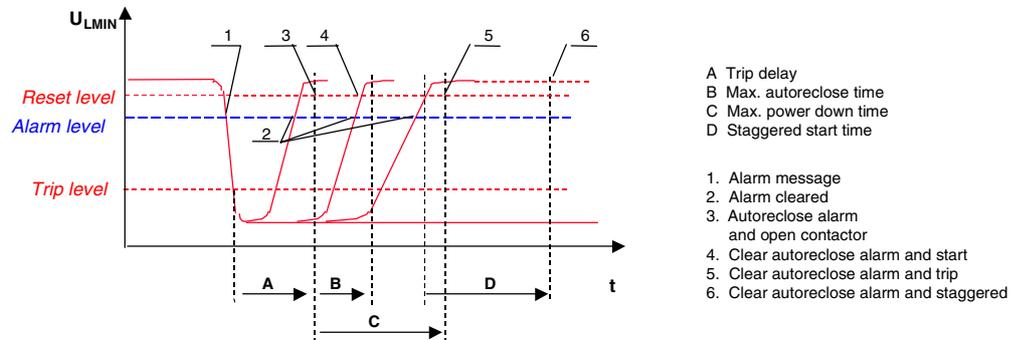
The lowest measured main voltage ( $U_{Lmin}$ ) is compared against the undervoltage *Alarm level*. When  $U_{Lmin}$  decreases below the undervoltage *Alarm level*, an “Undervoltage alarm” alarm is issued.
