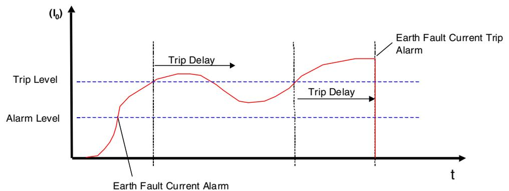
$I_0$  is compared against the earth fault current *Alarm level*. When  $I_0$  exceeds above the *Alarm level*, an "Earth Fault Current alarm" alarm is issued.
