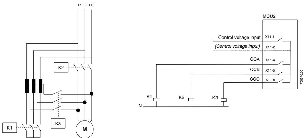
**Picture 34.** Control circuit for autotransformer starter, example 3.
