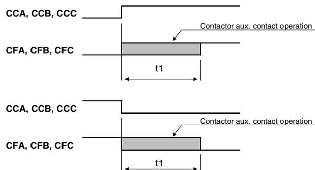
When enabled by parameterization, feedback supervision cyclically checks the contactor auxiliary contact statuses. If a difference between the control status and auxiliary status is detected, an alarm message is issued. If there is difference between control status and current measurement a trip message is issued and contactor is tripped as stated in the tables below.
