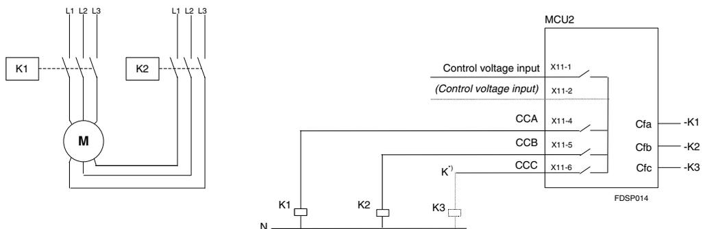
K<sup>3</sup> Feedback signal Cfc must be connected for feedback supervision.
