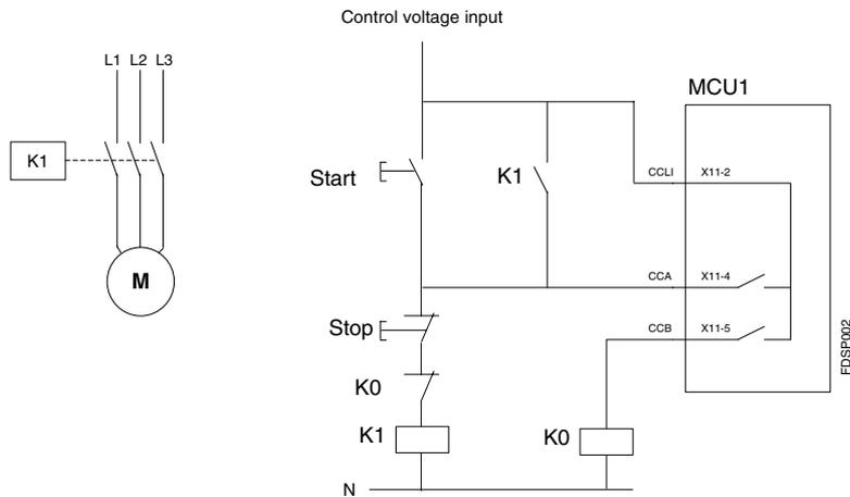
**Picture 20.** Control circuit for NR-DOL/RCU starter for MCU2.
