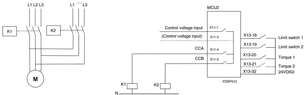
The use of torque switch is selected by setting the parameter for Actuator type, see table 37. Torque sensor can be connected to dedicated input. Torque switches are connected to inputs CFC (torque 1) and GPI1 (torque 2).
