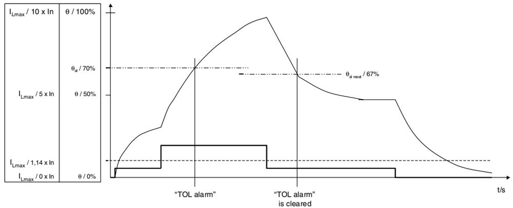
**4.2.4.5.4 Thermal protection overload alarm indication**
