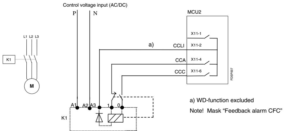
Latched contactor is parameterized separately and is available with starter types NR-DOL and REV-DOL.
