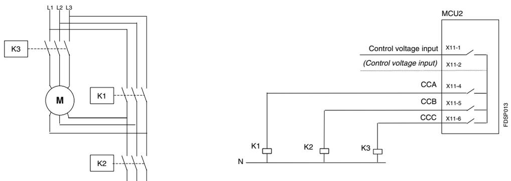
**Picture 26.** Control circuit for NR-2N with two contactors, separate windings, MCU2.
