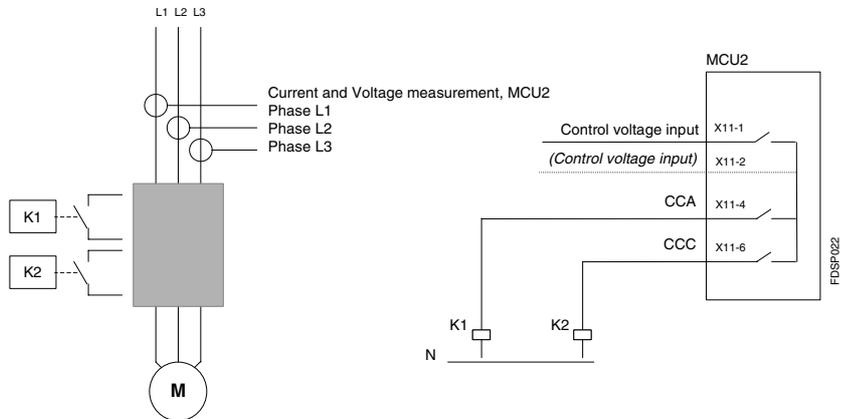
**Picture 16.** Control circuit with softstarter for REV-DOL, latched contactors.
