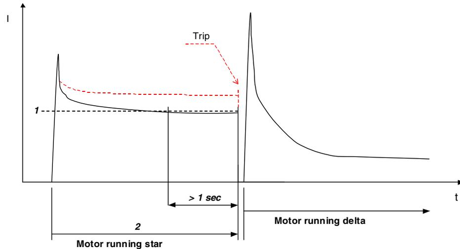
The MCU2 control contactors with sequence presented in the control logic picture. For all contactor conditions the previous condition must be fulfilled before a new control is executed (feedback supervision enabled). If feedback supervision activates a trip, the start will be cancelled accordingly.
