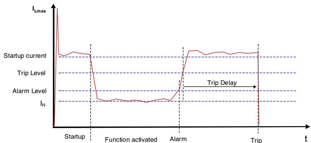
Stall function activates after the motor startup is completed (highest measured phase current  $I_{Lmax}$  decreases less than  $1.25 \times I_N$ ) or motor nominal startup time has elapsed.
