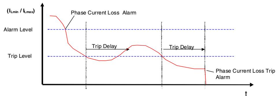
$I_{Lmin}/I_{Lmax}$  is compared against the phase loss *Alarm level* parameter. When  $I_{Lmin}/I_{Lmax}$  decreases below the *Alarm level*, an "Phase Loss alarm 1/2/3" alarm is issued.
