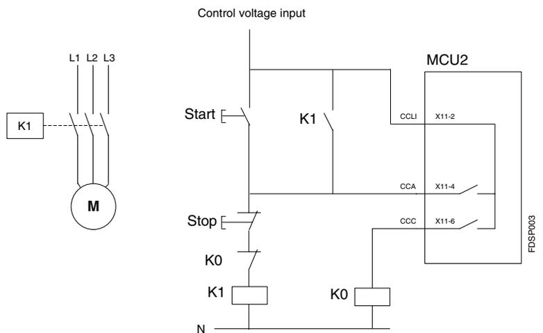
RCU-switch can be e.g. mom-off-mom type switch ('mom' stand for 'momentary on' with spring returning the switch to off position). On the other hand, RCU connection can also be done with normal switches as presented in example circuit on appendix section.
