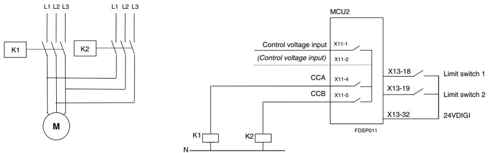
Limit switch causes the motor to be stopped when activated. Event message is sent to the fieldbus according to activated limit switch and additionally start command is allowed only to reverse direction.
