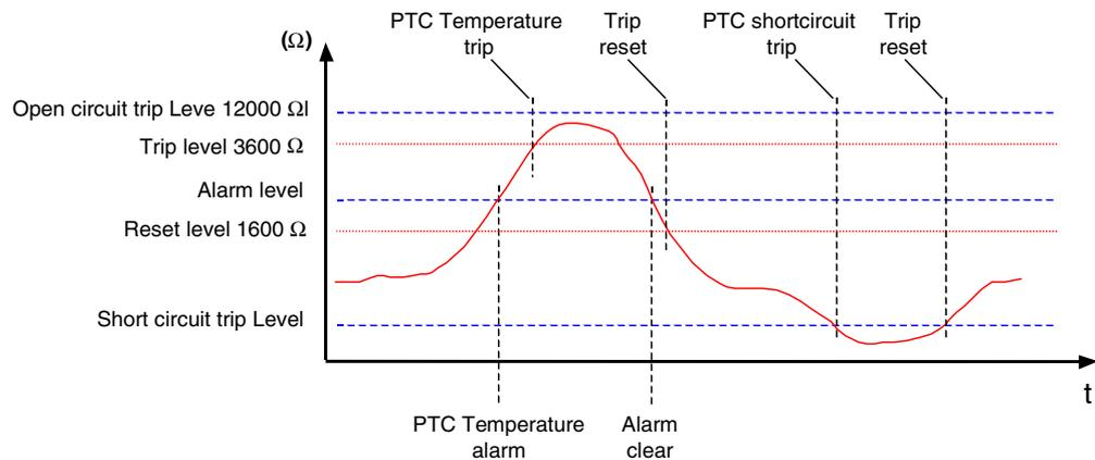
The resistance of PTC input is compared against the *Alarm level*. When resistance of PTC input exceeds above the *Alarm level*, an "PTC alarm" message is issued.
