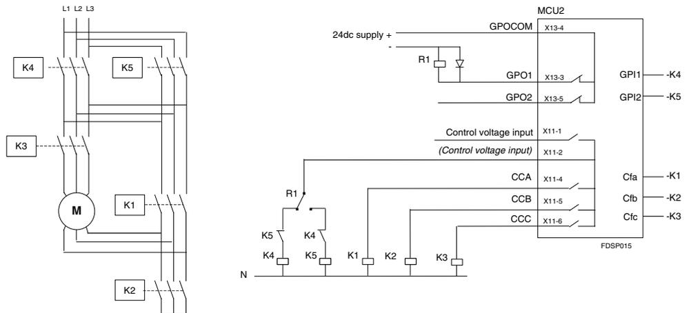
**Picture 29.** Control circuit for REV-2N starter with separate windings.
