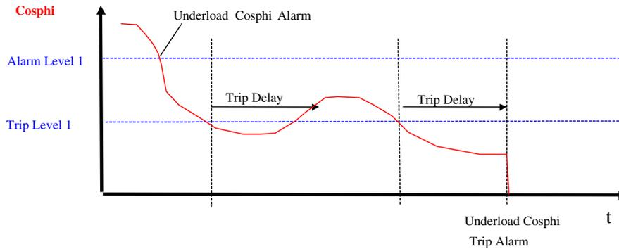
The cosphi value is compared against the underload cosphi *Alarm level*. When cosphi decreases below the *Alarm level*, an “U/L Cosphi alarm” alarm is issued.
