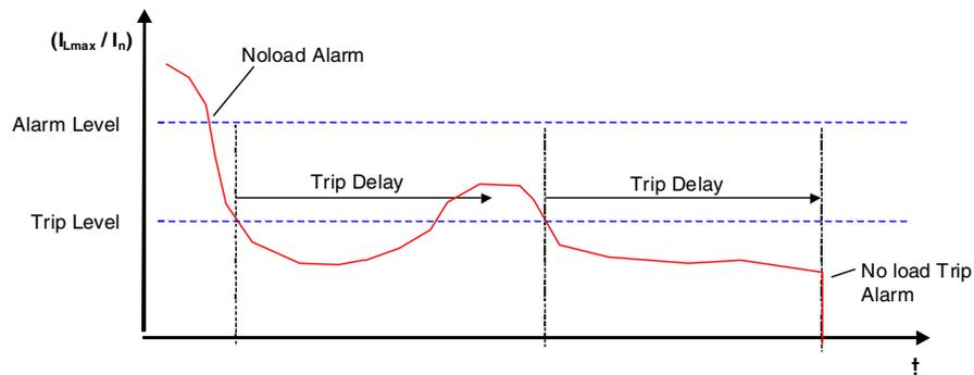
The highest measured phase current ( $I_{Lmax}$ ) is compared against the no load *Alarm level*. When  $I_{Lmax}$  decreases below the *Alarm level*, an “N/L alarm” alarm is issued.
