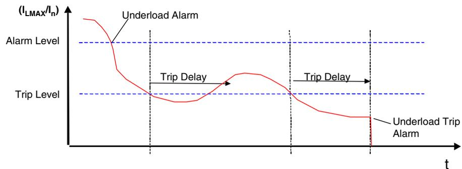
The highest measured phase current ( $I_{Lmax}$ ) is compared against the underload *Alarm level*. When  $I_{Lmax}$  decreases below the *Alarm level*, an “U/L alarm” alarm is issued.
