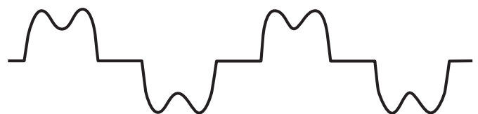
A voltage and current that deviate from the sine form contain harmonics.
