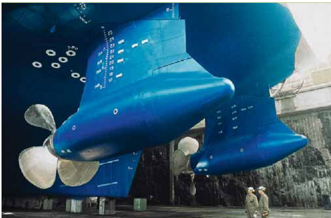
8 ABB's Azipod system for ship propulsion
