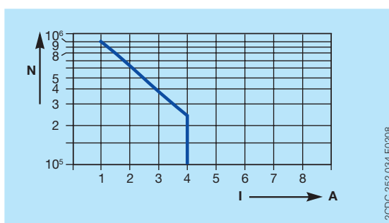
Contact lifetime /switching cycles N 220 V 50 Hz AC1, 360 cycles/h
