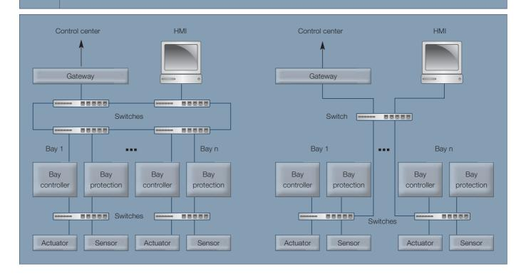
IEC 61850 communication can be seen as a two-level network comprising the process and the station level communication. Both concepts allow the networks to be combined, ie the IIT server and control networks may be the same physical LAN, just as the station and process level networks may be the same station-wide network. (Note that, since IEC 61850 covers the interoperable communication for the entire substation, it does not define the integration of field buses in any way.)
