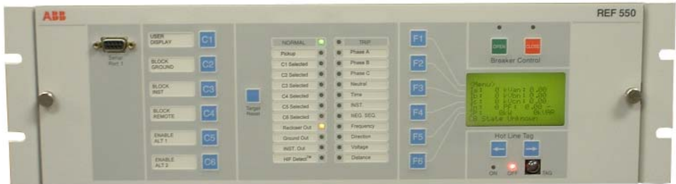
Figure 3-1. Front View of the OCI Panel with the Hot Line Tag Feature
