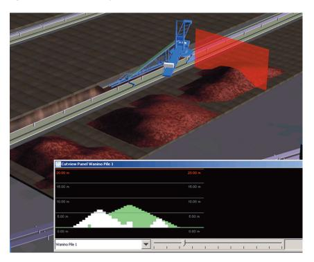
Figure 5. Selection of a cut view.
