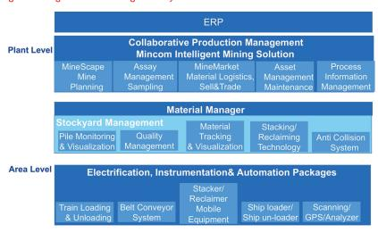
Figure 2. Modular system for bulk material handling.
