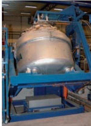
Left picture: Simulation tools are based on 1200 EMS installations and quickly indicate a possible solution, project payback and performance guarantee. At Ljunghäll AB the result is effective stirring of the entire melt, ~1 rotation/minute.
