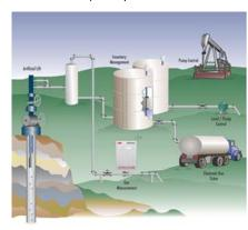
the gas sales valve and the blow valve is achieved as the XSeries monitors several well parameters to provide inputs to a Continuous Control Tuning Algorithm. This algorithm is the key element in optimized plunger operation.
