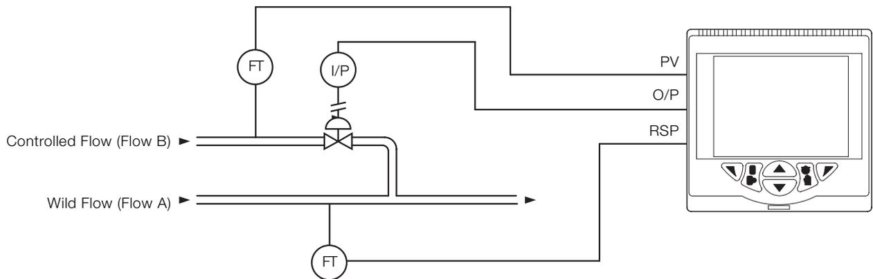
Fig. 21: Ratio controller
