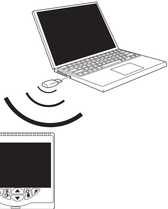
Fig. 16: Transferring a configuration file via the infrared port
