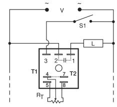
Dashed lines are internal connections.  $R_{\tau}$  = 100 K $\Omega$  S1 = Optional Low Current Initiate Switch T1 = ON Time T2 = OFF Time
