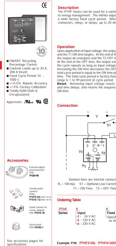
The PTHF Series can be used for a variety of applications from chemical metering, to temperature regulating, to energy management. The infinite adjustability from 1 to 99% provides accurate percentage ON control over a wide factory fixed cycle period. When mounted on a metal surface, it can be used to drive solenoids, contactors, relays, or lamps, up to 20 Amps steady, 200 Amps inrush.
