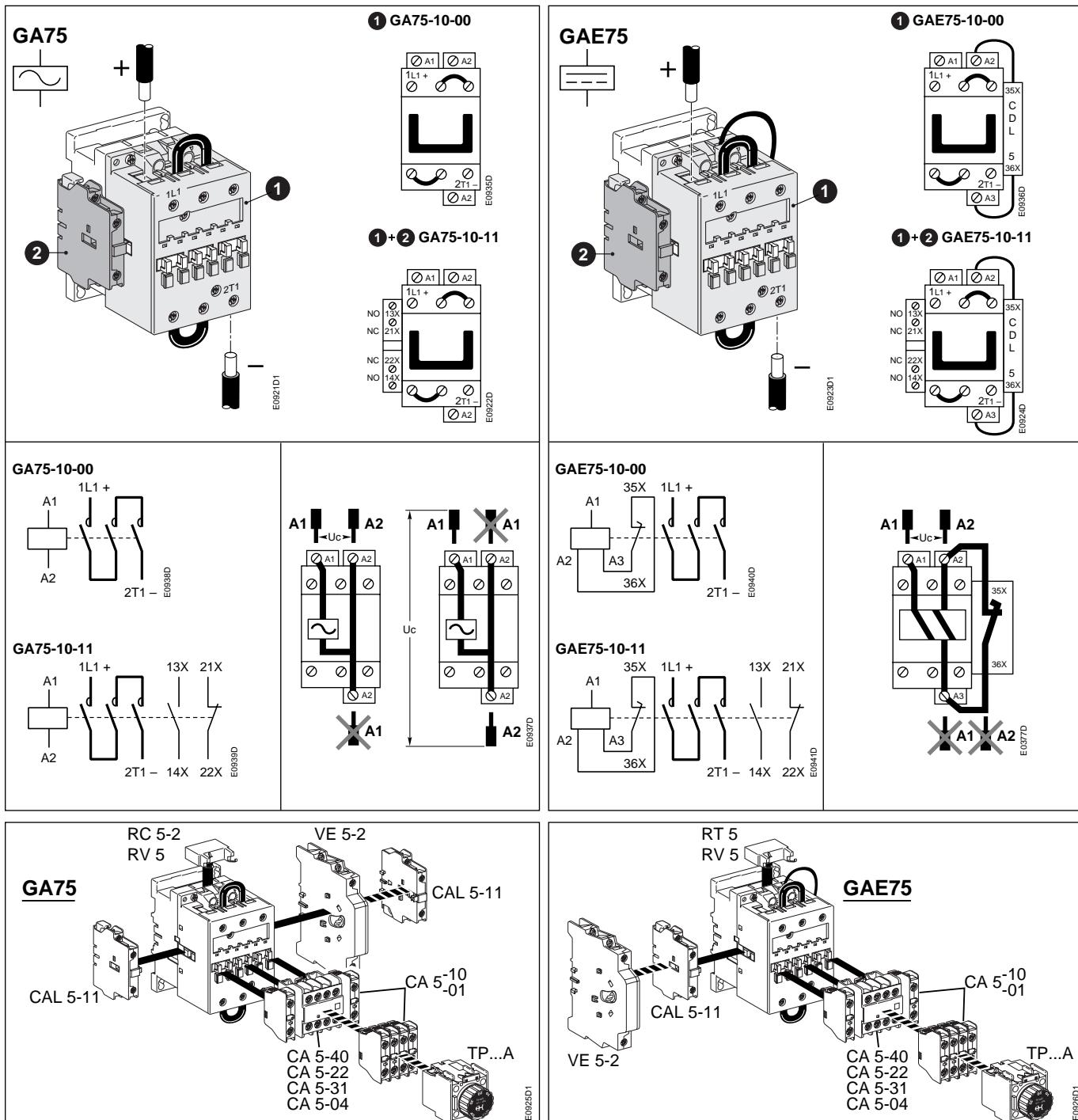
**Warning !** The operation, installation and servicing of this appliance must be carried out by a qualified electrician applying the relevant rules of the art, installation standards and safety regulations. Before operating the contactors, check that control voltage complies with the data on the coil mounting bracket. Connection to other control voltage can destroy the coil. Do not touch live parts. Danger !
