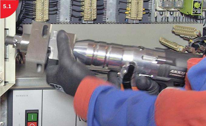
Rotate the cutting head to set the correct cutting direction.
