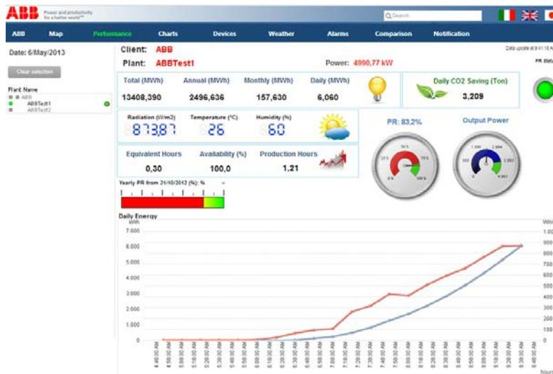
Figure 11: Typical real-time cockpit for current production level and relevant KPI's.
