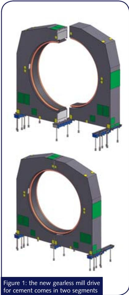
Figure 1: the new gearless mill drive for cement comes in two segments
