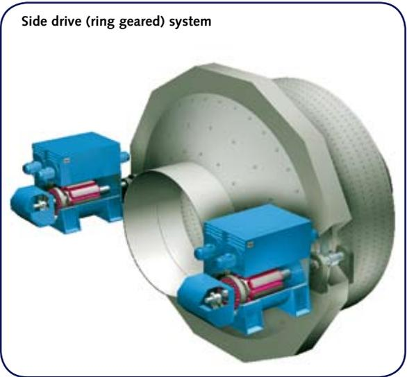
Figure 6: torque transfer happens through the pinion which inherently produces friction losses and requires regular lubrication and alignment to avoid premature failure. To run the mill at slow speeds ie, to replace liners, either a variable speed mill drive system or an additional auxiliary drive is required
