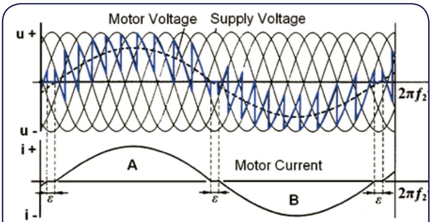
Figure 4: operating principle of a cyclo converter: the motor voltage is generated directly from the supply voltage
