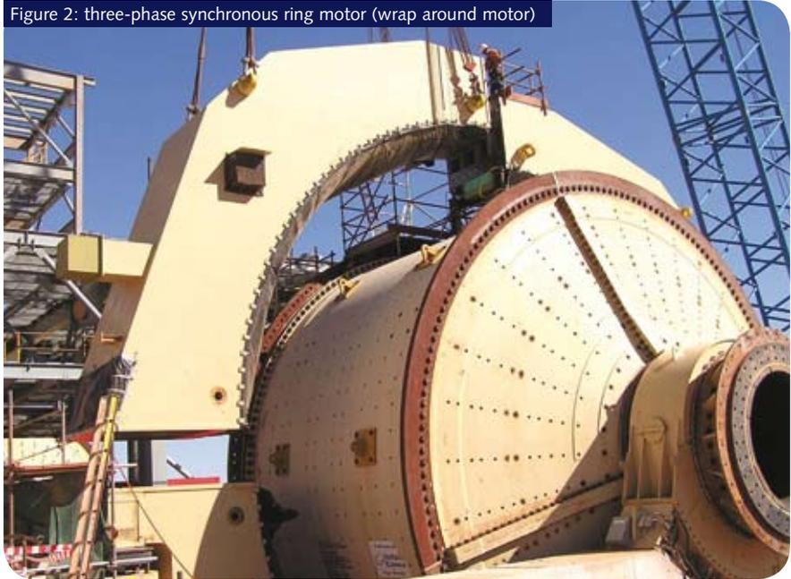
Figure 2: three-phase synchronous ring motor (wrap around motor)
