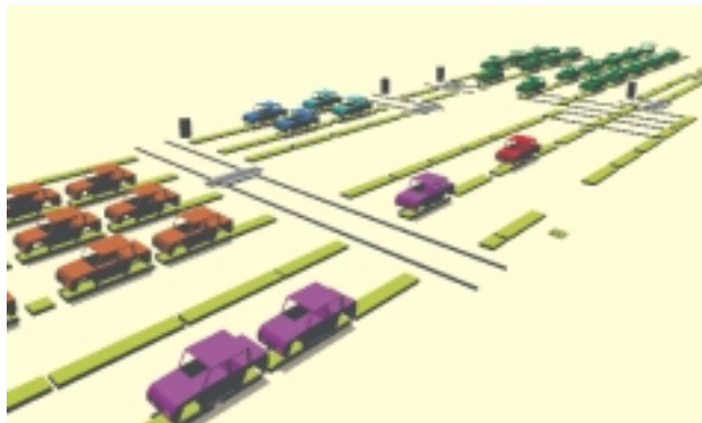
Simulation of a complete paint finishing line: level 1 with inspection, repair and buffer areas
