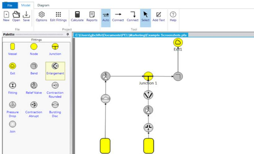
PEL ADRIAN calculates flows and pressures for high velocity, compressible gases in a network and is relevant for the modelling of relief streams
