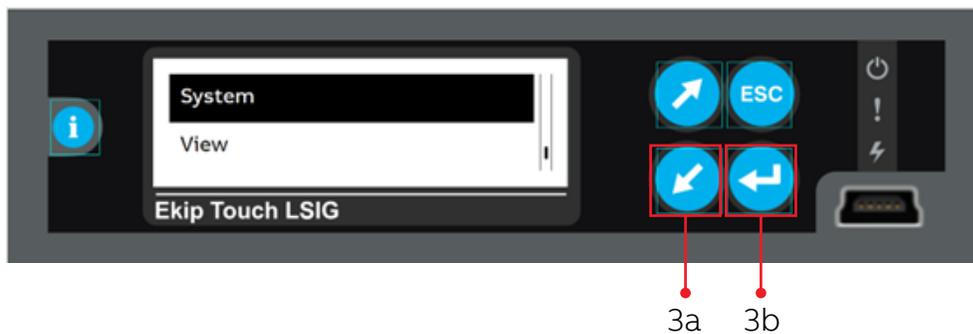
Step 4. Press **Down** button (4a) to find **Date** menu and Press **Enter** button (4b).
