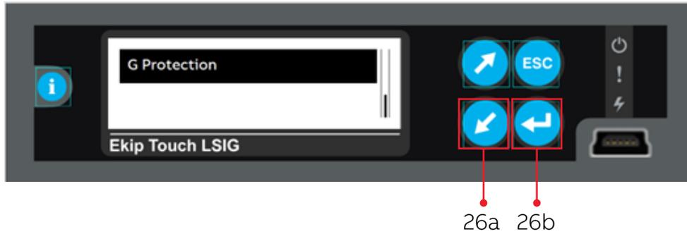
Step 27. Press Enter button (27) to Enable G Protection.
