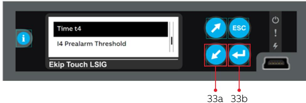
Step 34. Change the **Ground Fault Time Delay / Time t4** setting to the value in the coordination study using the **Up** or **Down** buttons (34a) and Press **Enter** button (34b).
