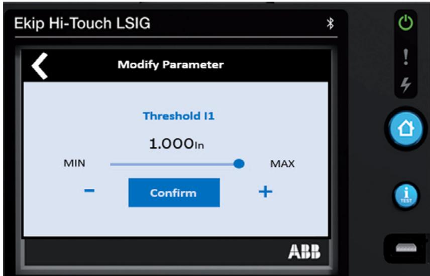
The setting range is from 0.4 to 1.0 of the breaker's nominal rating (rating plug value)
