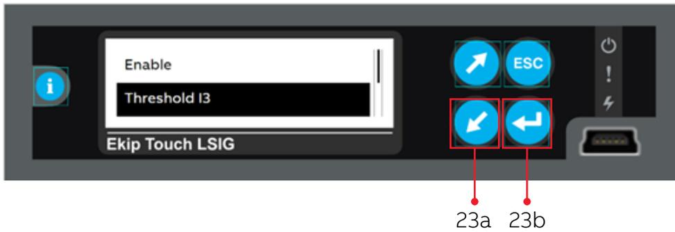
Step 24. Change the **Instantaneous Pickup / Threshold I3** setting to the value in the coordination study using the **Up** and **Down** buttons (24a) and Press the **Enter** button (24b).
