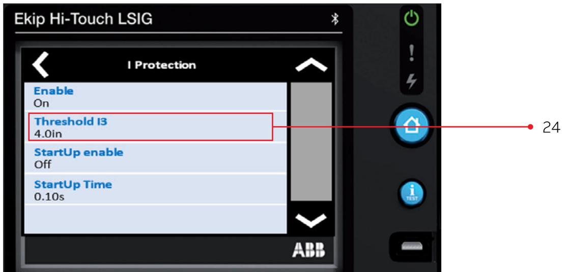
Step 25. Change the **Instantaneous Pickup / Threshold I3** setting to the value in the coordination study.
