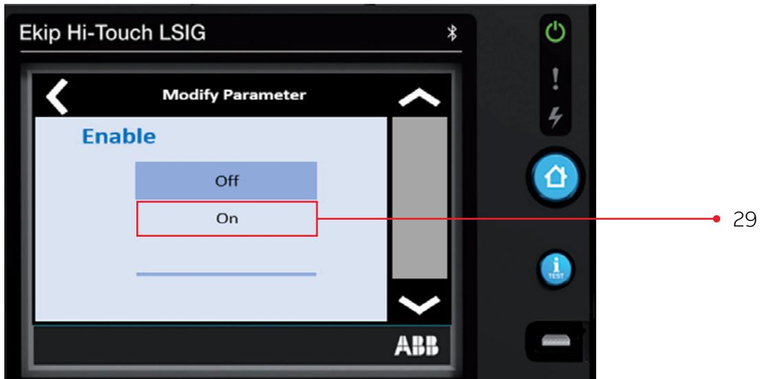
The Ground Fault - **G Protection** Function is now Enabled
