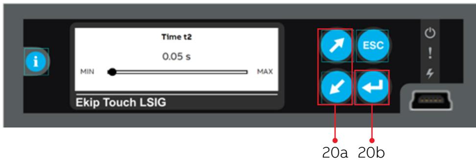
The setting range is from 0.05 to 0.8 Seconds (UL Version: t4 Max = 0.4s)
