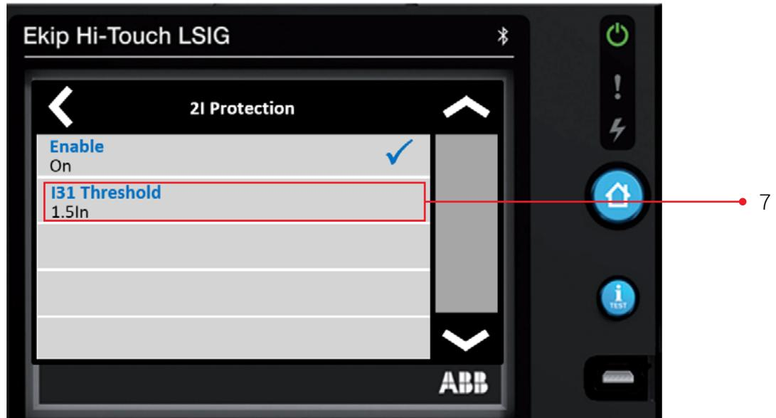
Step 8. Change the **Arc Flash Mitigation / RELT / I31 Threshold** setting to the value in the coordination study.
