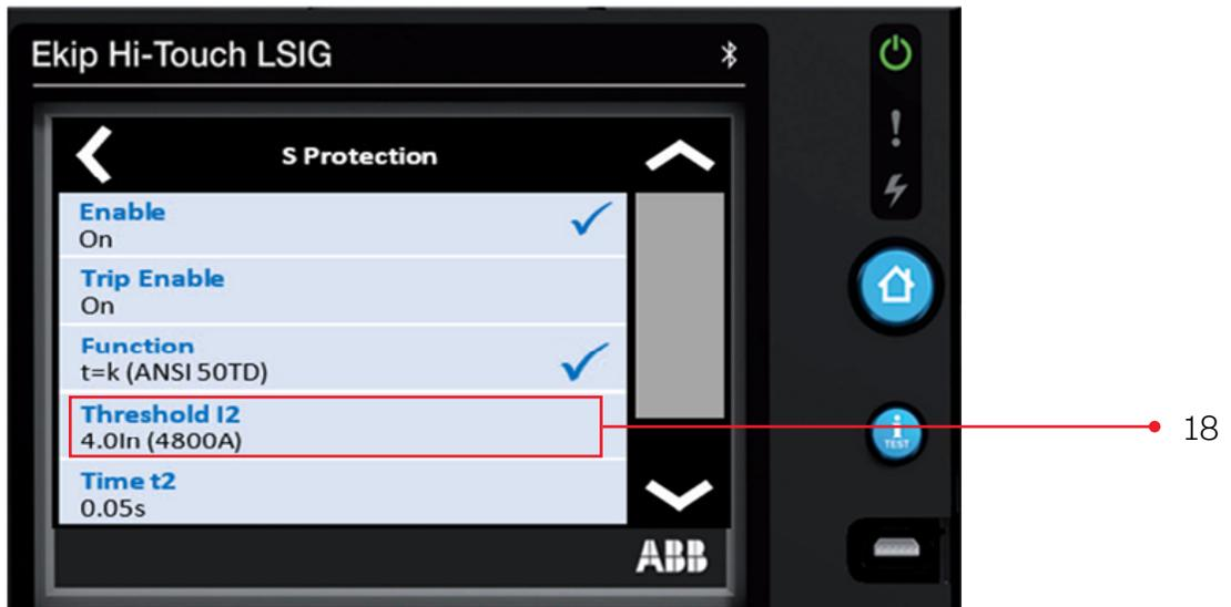
Step 19. Change the **Short Time Pickup / Threshold I2** setting to the value in the coordination study.
