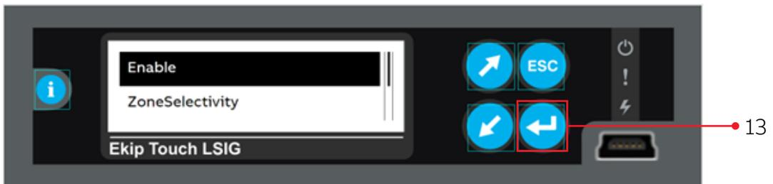
Step 14. Press **Down** button (14a) to **On** and press **Enter** button (14b)
