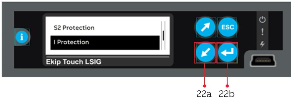
Step 23. Press **Down** button (23a) to select **Threshold I3** and Press **Enter** (23b).
