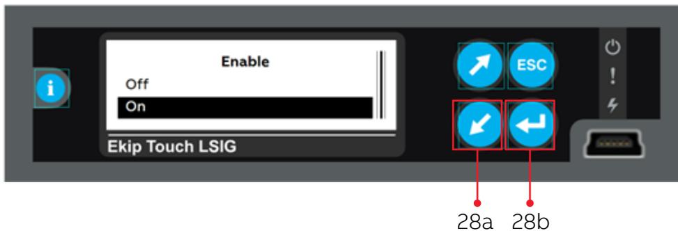
The Ground Fault – G Protection Function is now Enabled
