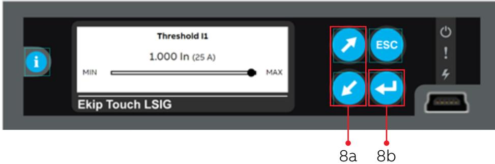
The setting range is from 0.4 to 1.0 of the breaker’s nominal rating (rating plug/sensor value) Press **Up** or **Down** buttons (8a) to change to the value in the coordination study. Then Press **Enter button** (8b) and this screen will be displayed.
