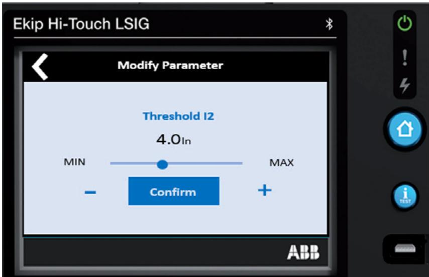
The setting range is from 0.6 to 10.0 of the breaker’s nominal rating (rating plug value)
