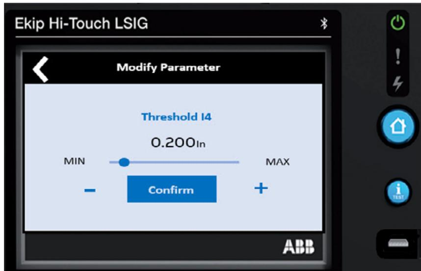
The setting range is from 0.1 to 1.0 of the breaker's nominal rating (rating plug value) (UL Version: I4 Max = 1200A)
