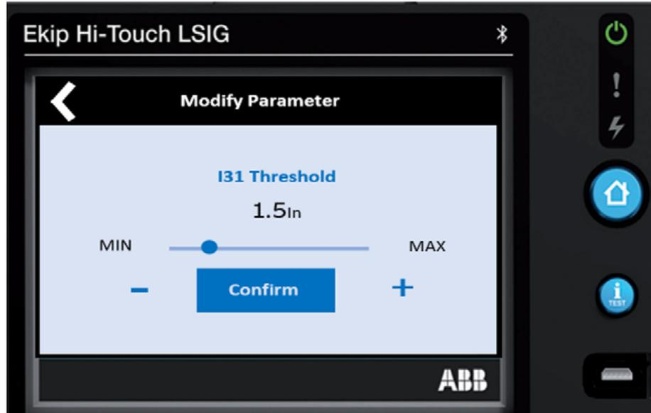
The setting range is from 1.5 to 15.0 of the breaker's nominal rating (rating plug value). Press the **minus icon** or the **plus icon** to change to **the value in the coordination study** (maintaining the press will advance the settings faster). Then press **Confirm**.
