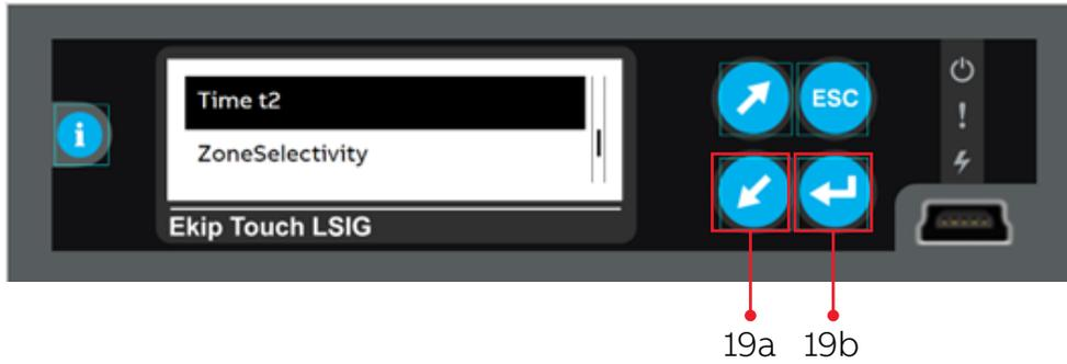
Step 20. Change the **Short Time Delay / Time t2** setting to the value in the coordination study using the **Up** and **Down** buttons (20a) and Press the **Enter** button (20b).
