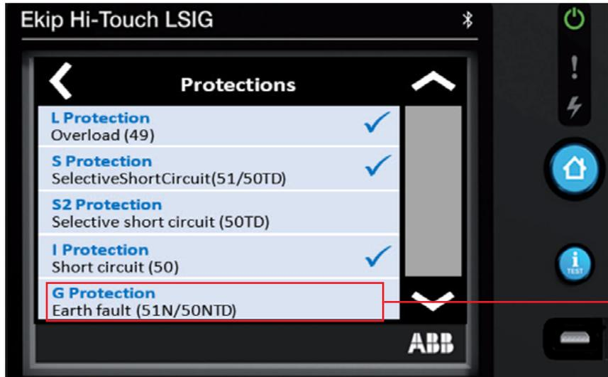
NOTE: For breakers using external neutral CT for ground fault protection change the breaker configuration from 3P to 3P + N. Go to Settings>Circuit Breaker>Configuration>Enter password 00001>3P + N>Home Button>Confirm
