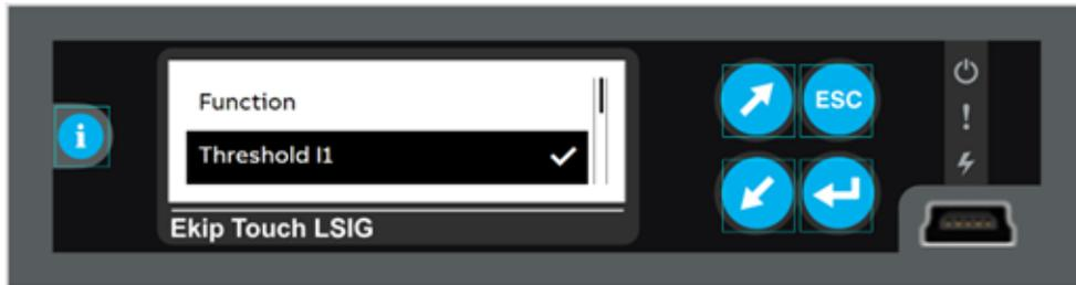
NOTE: The value is given as both absolute value (in Amperes) and relative value (In) and can be set within the range: 0.4 In to 1.0In in 0.001 steps
