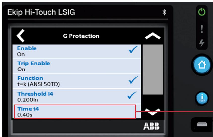
Step 35. Change the **Ground Fault Time Delay / Time t4** setting to the value in the coordination study.
