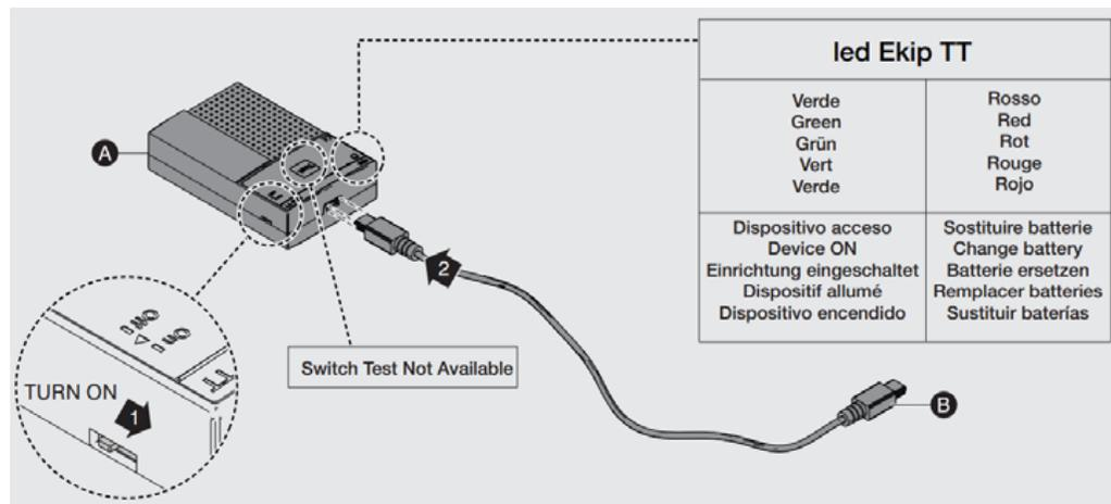
Step 1. Insert the **Ekip TT Plug End (B)** into Ekip Touch Trip Unit Service Connector (7)
