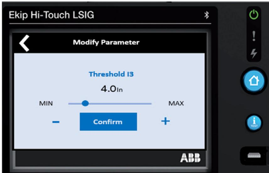
The setting range is from 1.5 to 15.0 of the breaker's nominal rating (rating plug value)
