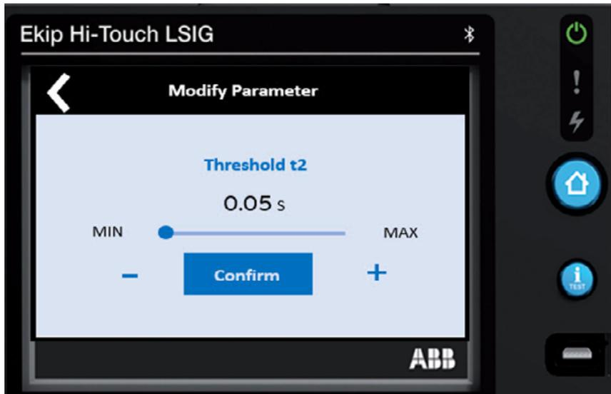
The setting range is from 0.05 to 0.8 Seconds (UL versions: t2 Max = 0.4s)
