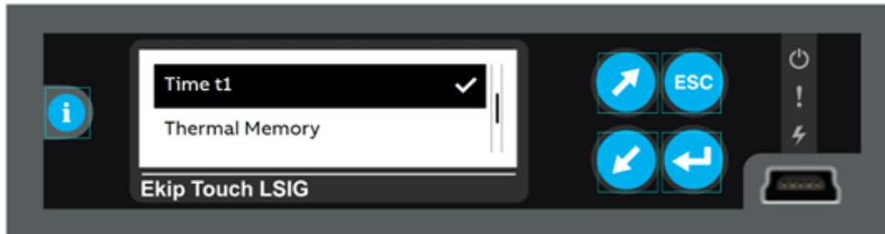
NOTE: The value is given in seconds and can be set within the range: 3 seconds to 144 seconds, in 1 second steps.
