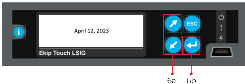
Step 7. Press **Down** button (7a) to select **Time** and Press **Enter** (7b).
