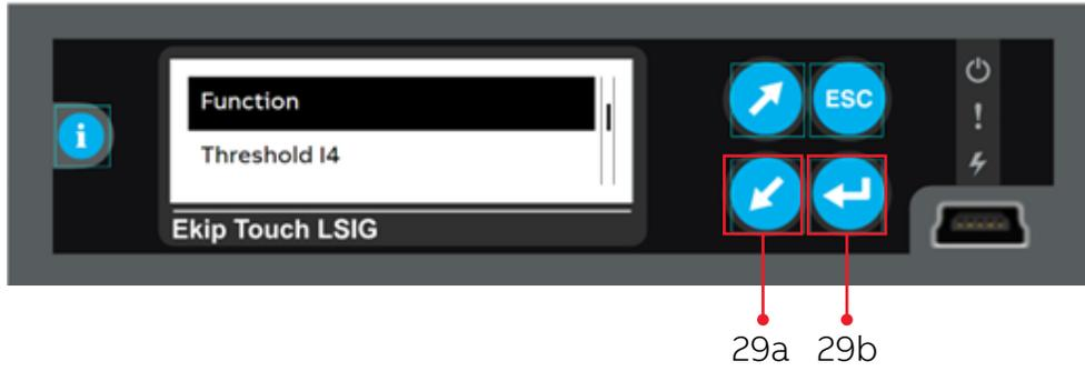
Step 30. Press **Down** (30a) and/or **Enter** (30b) to selection Function/Curve per coordination study.
