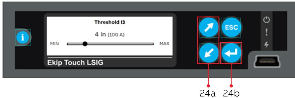
The setting range is from 1.5 to 15.0 of the breaker's nominal rating (rating plug/sensor value)
