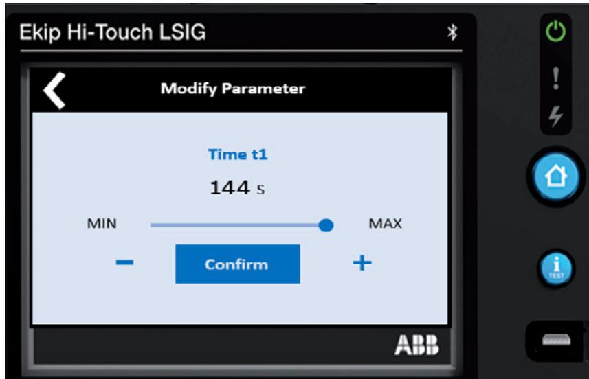
The setting range is from 3 to 144 Seconds (3 to 48 seconds for XT5)
