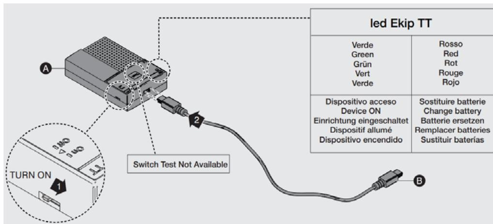
Step 1. Insert the **Ekip TT Plug End (B)** into **Ekip Touch Trip Unit Service Connector (G)**
