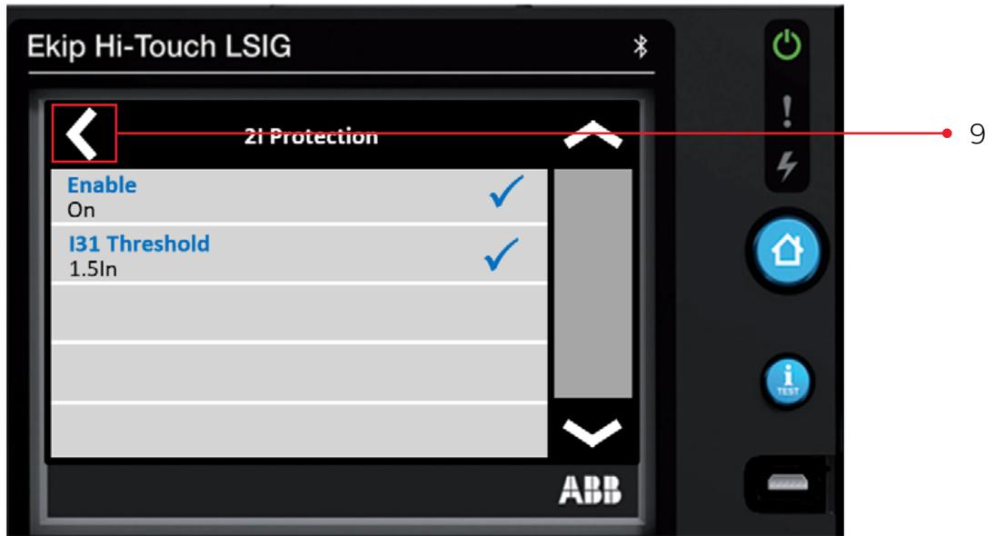
This completes the settings of the **Arc Flash Mitigation / RELT / 2I Protection** Function.
