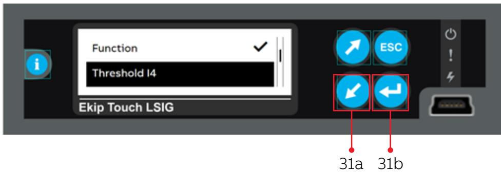
Step 32. Change the **Ground Fault Pickup / Threshold I4** setting to the value in the coordination study using the **Up** and **Down** buttons (32a) and Press the **Enter** button (32b).
