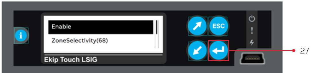
Step 28. Press **Down** button (28a) to select **Enable=ON** and Press **Enter** button (28b).
