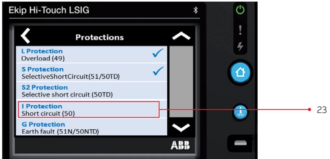
**ADJUSTING THE INSTANTANEOUS PICK UP OR THRESHOLD I3**
