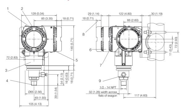
1 Adjustments | 2 Identification plate | 3 Certification plate | 4 Process connection | 5 Terminal side | 6 Integral display housing | 7 Electronic side | 8 Space for cover removal | 9 Drain/vent valve
