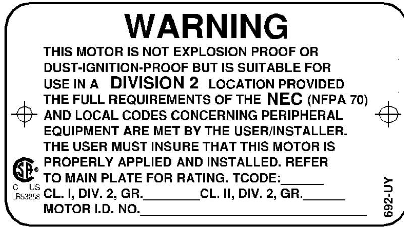
Figure 2 Example nameplate for machines manufactured according to CSA hazardous area
