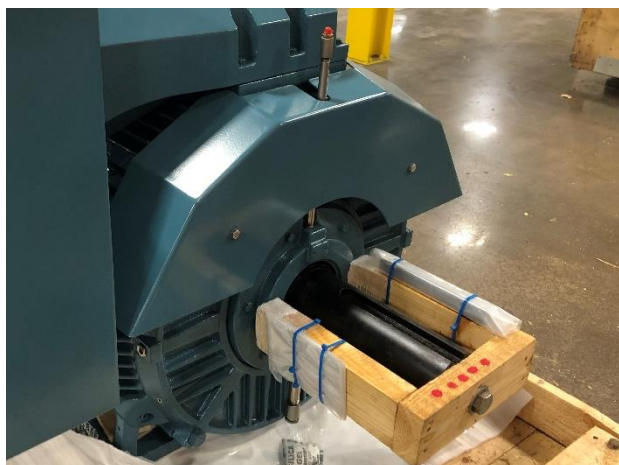
Figure 15 Option 1 – wooden rotor locking device
