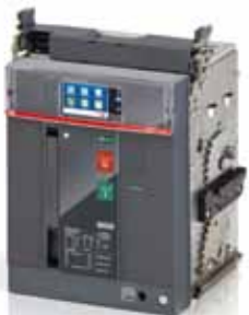
E2.2H 1600A, 3 poles, moving part with Ekip G Hi-Touch
