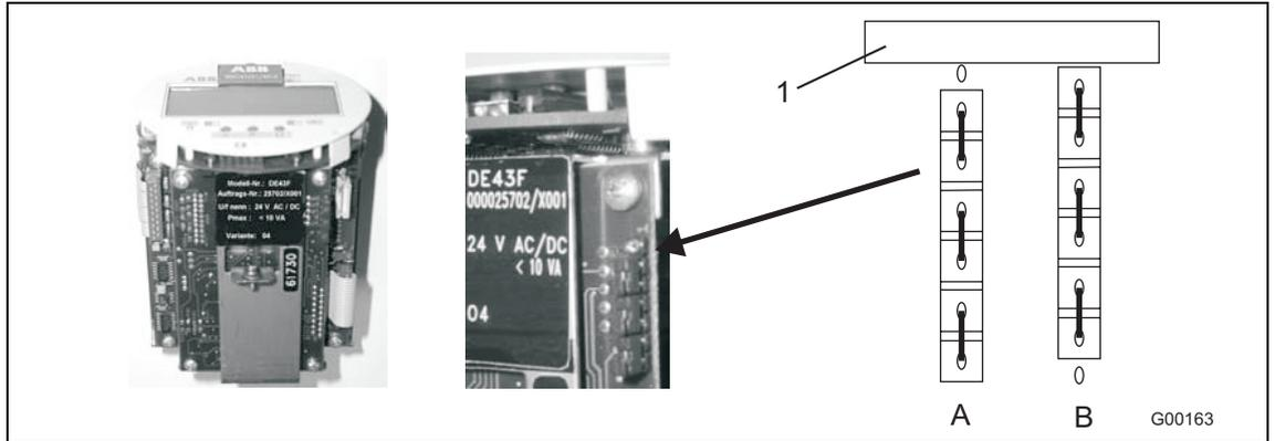
Fig. 28 Setting the pulse output using jumpers
