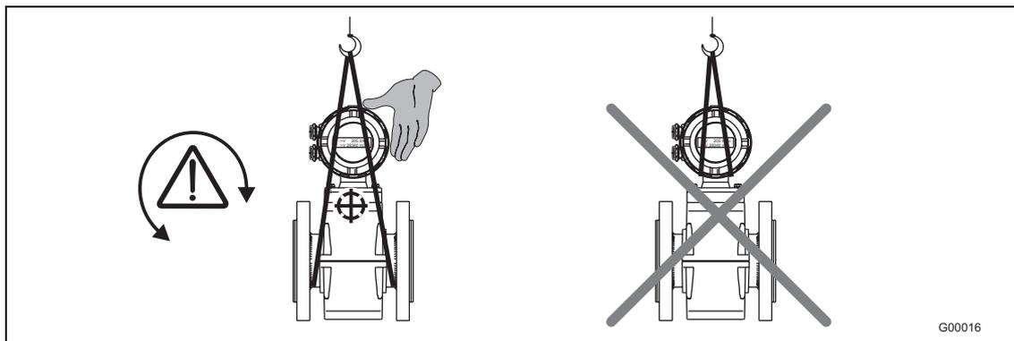
Fig. 1: Transport of flanged units smaller than DN 450
