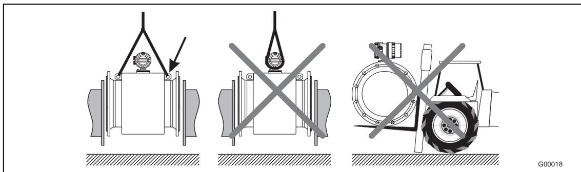
Fig. 2: Transport of flanged units larger than DN 400
