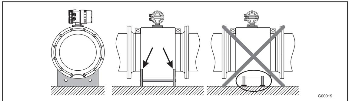
Fig. 10: Support for meter sizes larger than DN 400
