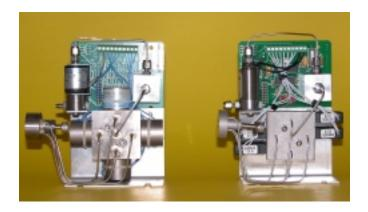
The Model 8000 design has been unique in that it has very few moving parts and as such is the most dependable and easiest to start up of any on-line GC on the market. The SSM, having 4 electric solenoids has been the most likely part to fail just due to the concentration of moving mechanical parts. This change should make even this portion of the Btu Transmitter even more reliable than before.
