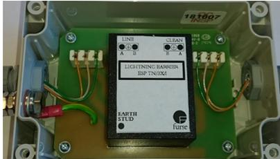
Figure 4. IDC connection option (suffix /I)
