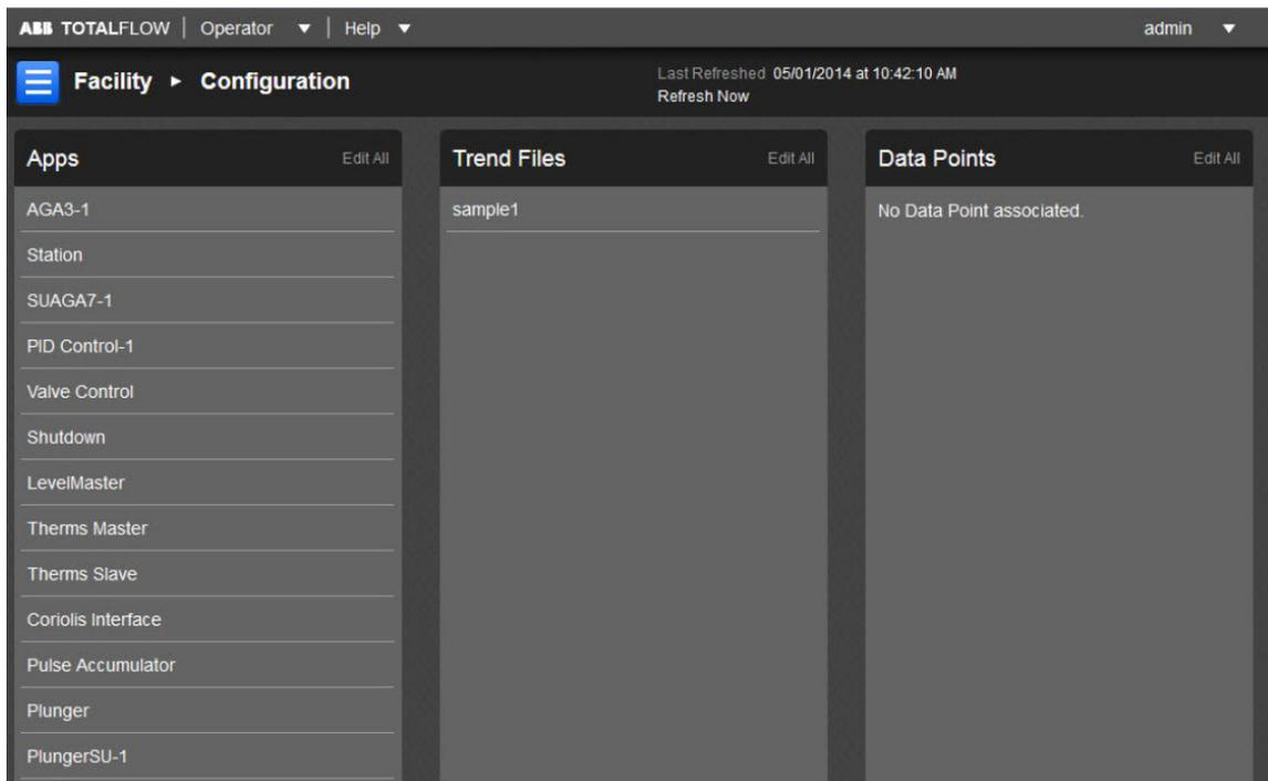
On opening the well sections and/or the facility section, there are three tabs that the user can select from: Apps, Trend Files, and Data Points.
