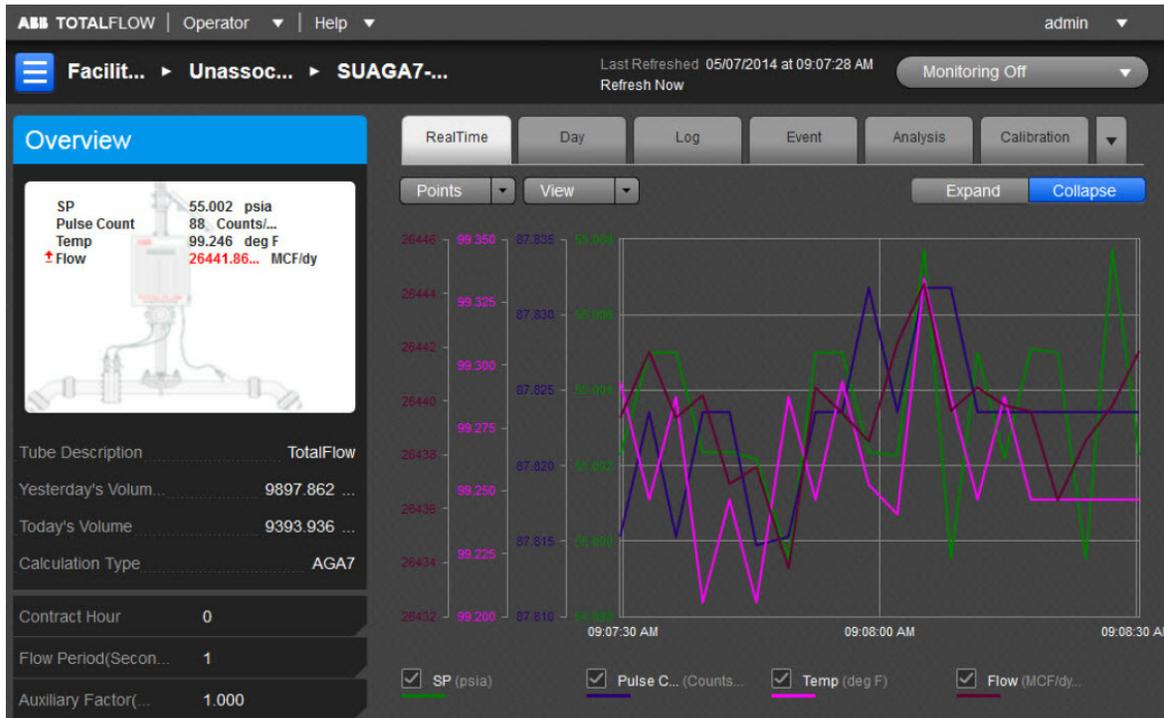
The user can also use the general information displayed as a snapshot of the current existing values for each parameter listed. There can be up to eight (8) AGA-7 measurement applications instantiated per comm channel on the XFCG4 board. The fields displayed here are as follows:
