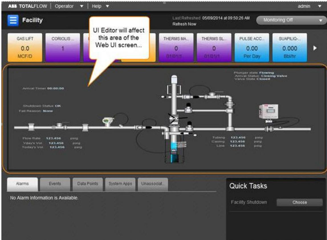
If the Site Map is not loaded in the device, the regular production data is displayed including the graph and tank information. In the upper left corner of the production display is the SVG icon. Using this icon, the user will receive an error message if trying to call up the production display (graph). If the Site Map is loaded, selecting the SVG icon will display the UI Editor.
