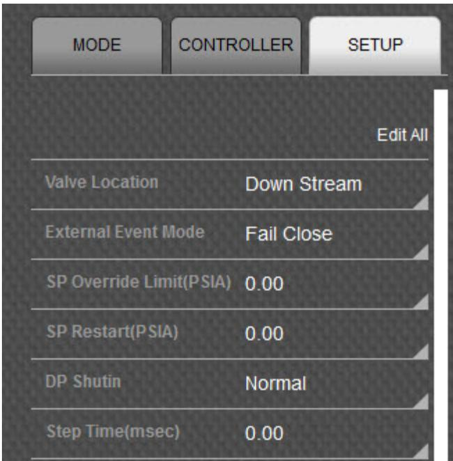
The following will detail the parameter fields that the user can expect to encounter within the Setup tab:
