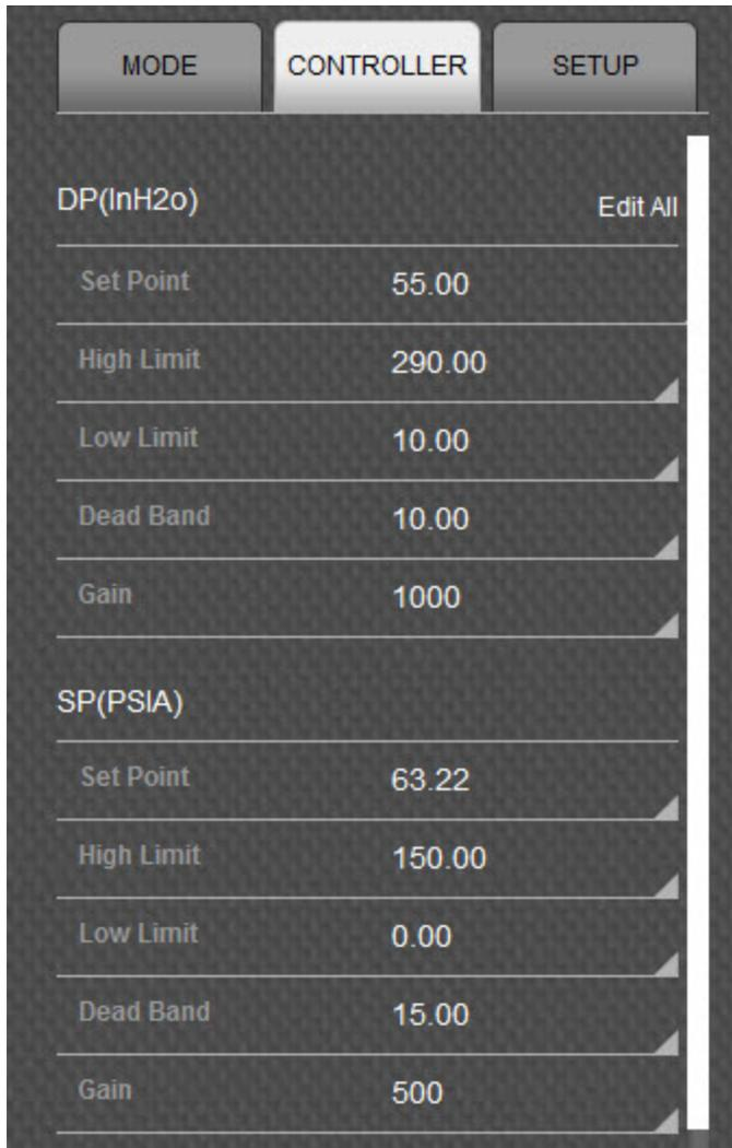
The following will detail the parameter fields that the user can expect to encounter within the Controller tab. Depending on what the user elects to use as the Control method (DP, SP or Flow Rate), the parameter fields are the same, regardless of which Control method is selected.
