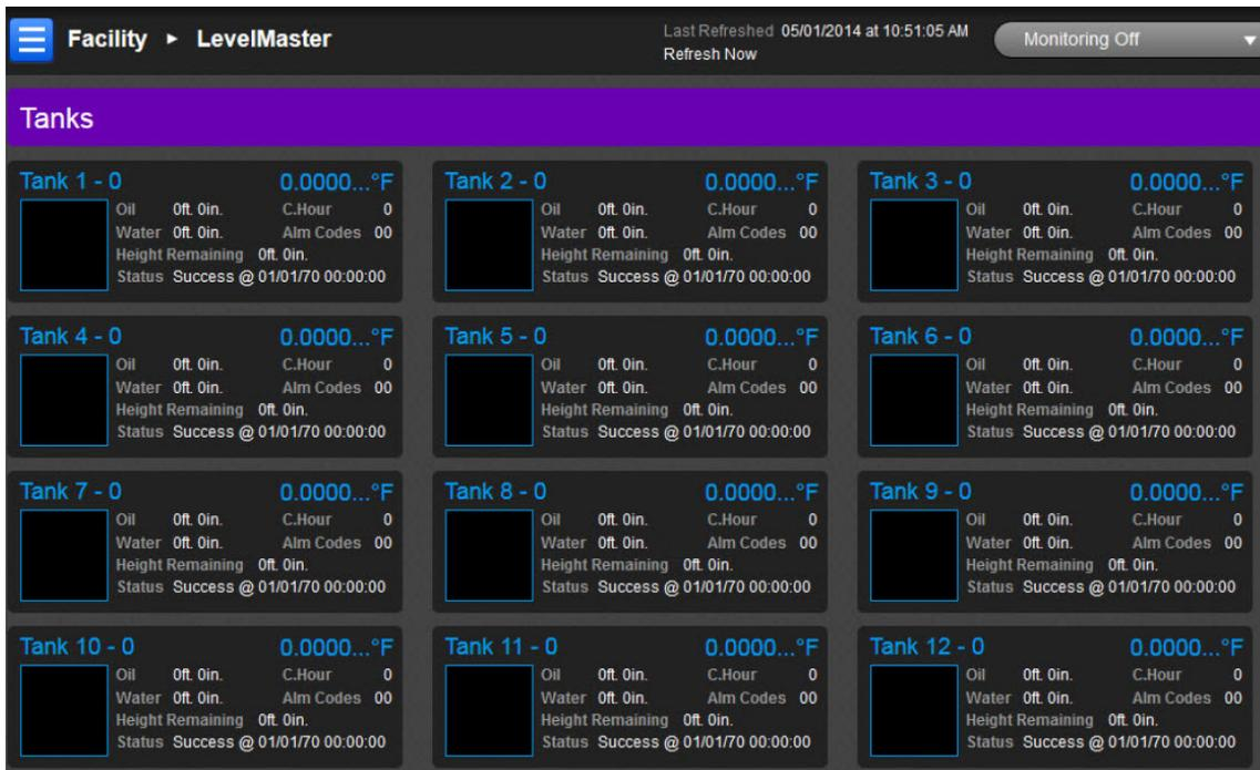
Depending on the number of tanks that the user has established in PCCU32, the user sees up to 15 tanks displayed within the Tanks section on the Facility Dashboard. Here on the Tanks application screen all the tanks can be displayed. Each tank is treated as its own individual unit, and the user can see composite information regarding that individual tank. This also includes alarm indications (note tanks 1-0, 3-0 and 4-0).
