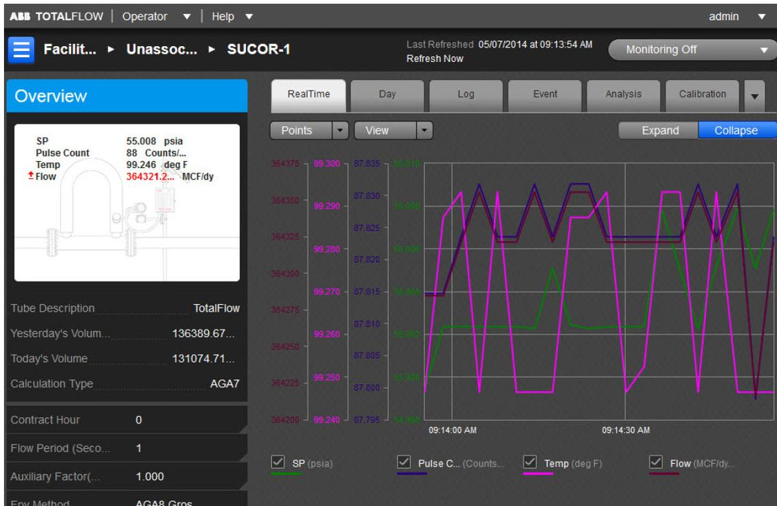
The user can also use the general information displayed as a snapshot of the current existing values for each parameter listed. There can be up to eight (8) SUAGA-7 measurement applications instantiated per comm channel on the XFCG4 board. The fields displayed here are as follows:
