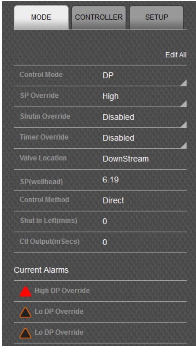
The following will detail the parameter fields that the user can expect to encounter within the Mode tab:
