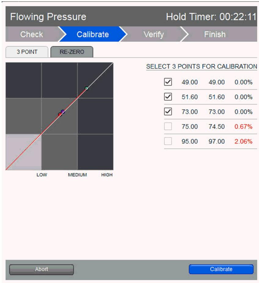
If the user chooses to calibrate, the Calibrate screen will display with the points plotted and listed in a table. If a 3-point calibration had been selected in setup but had done more than three checks, the user would have the option to check the boxes of desired points to use for the calibration. If however, a 3-point calibration was set up and three checks were done, naturally there is no option. Click the Calibrate button to continue.
