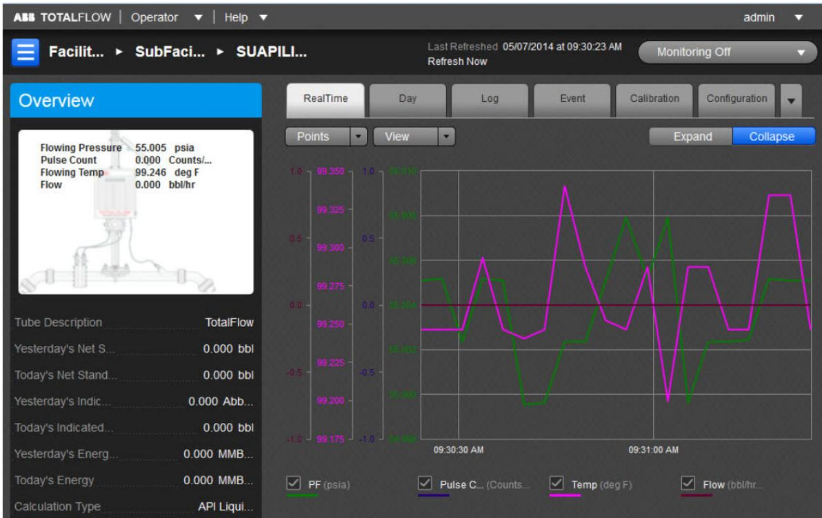
The user can also use the general information displayed as a snapshot of the current existing values for each parameter listed. There can be up to eight (8) SULiquid measurement applications instantiated per comm channel on the XFCG4 board. The fields displayed here are as follows:
