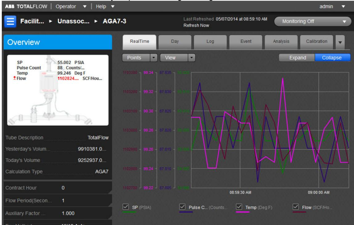
The user can also use the general information displayed as a snapshot of the current existing values for each parameter listed. There can be up to eight (8) AGA-7 measurement applications instantiated per comm channel on the XFCG4 board. The fields displayed are as follows:
