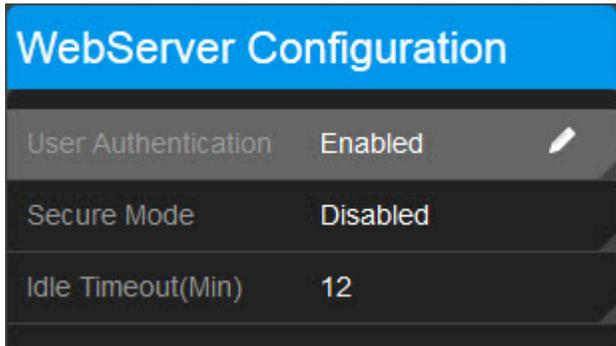
The system administrator can select User Authentication, Secure Mode and/or Idle Timeout (Min). Each of these sections can be edited by clicking on the Pencil icon. This brings up a corresponding dialog box where changes can be made to that particular section.
