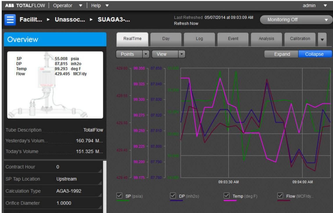
The user can also use the general information displayed as a snapshot of the current existing values for each parameter listed. There can be up to eight (8) AGA-3 measurement applications instantiated per comm channel on the XFCG4 board. The fields displayed here are as follows:
