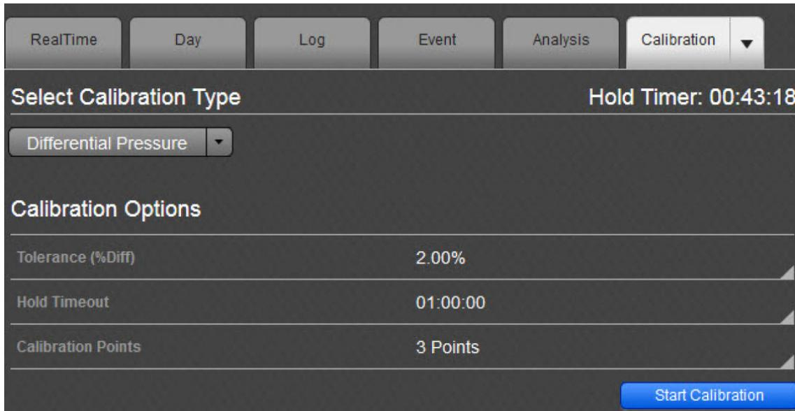
Next select the Differential Pressure Calibration Check and modify the read/write fields if necessary. Then click the Start Calibration to begin. Again the tube goes into the Hold state and the hold timer value for that tube is displayed on the right corner of the tab (defaults to 3600 seconds or one hour).
