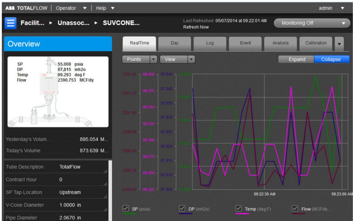
The user can also use the general information displayed as a snapshot of the current existing values for each parameter listed. There can be up to eight (8) V-Cone measurement applications instantiated per comm channel on the XFCG4 board. The fields displayed here are as follows:
