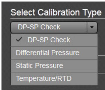
To start the calibration, select the type. Note the display of the Calibration Options fields changes depending on the calibration type selected as follows:
