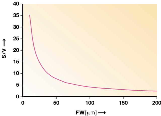
**11** Normalized surface-to-volume ratio (S/V) versus feature width (FW) for a corrugated fuel cell
