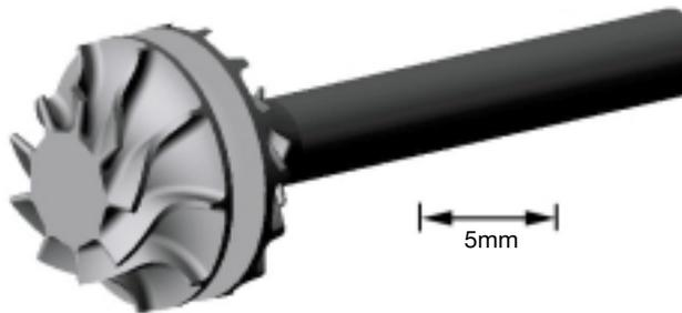
**7** The sintered micro-turbine used for the spin test
