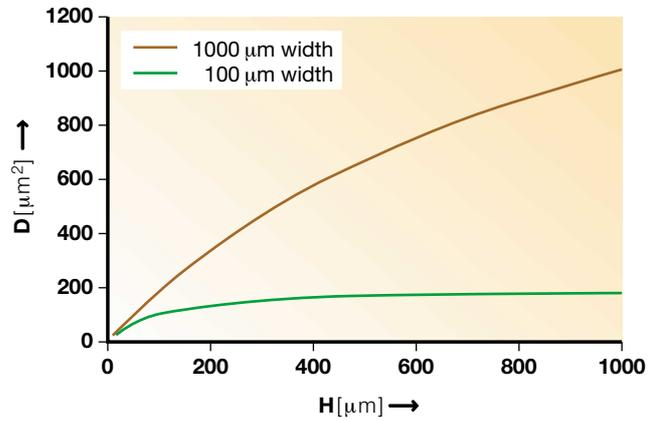
**12** Hydraulic diameter (D) versus channel height (H) for 2 channel widths.
