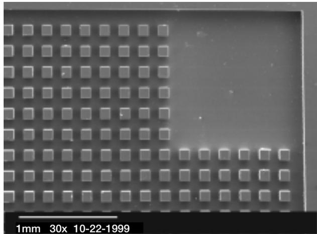
**16** Micro-porous electrodes produced by metal gel-casting
