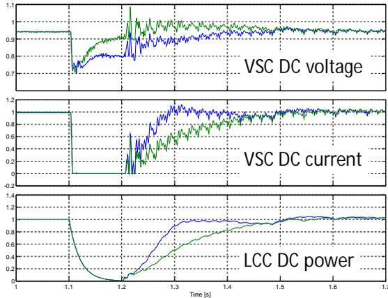
Figure 3, LCC 3-phase to ground AC fault, Mode 2
