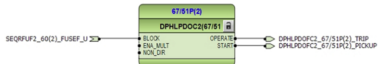
Figure 42: Three phase Directional overcurrent protection - LV side
