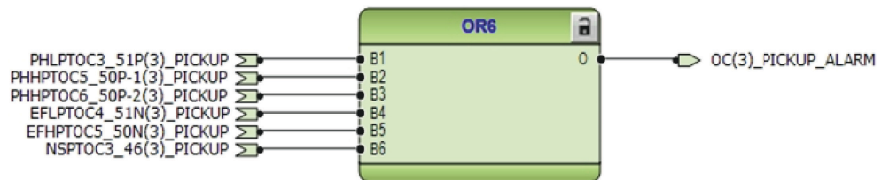
Figure 107: Overcurrent pickup alarms - Tertiary side
