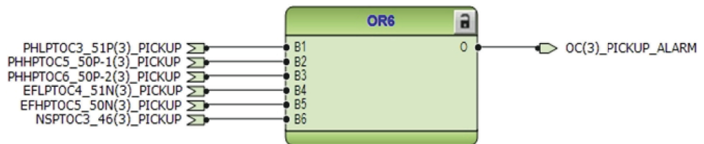
Figure 51: Overcurrent pickup alarms - Tertiary side
