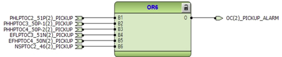
Figure 106: Overcurrent pickup alarms - LV side
