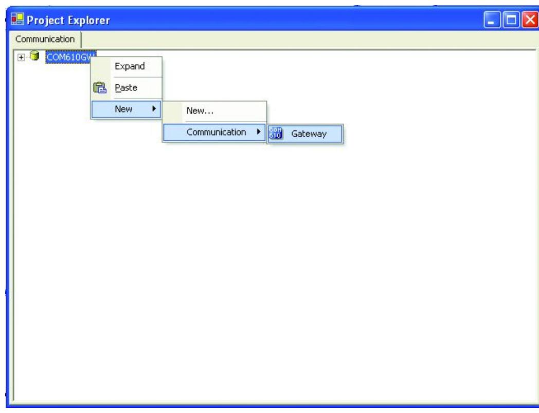
*Figure 3.2.2-1 Adding a COM610/615 Gateway object*
