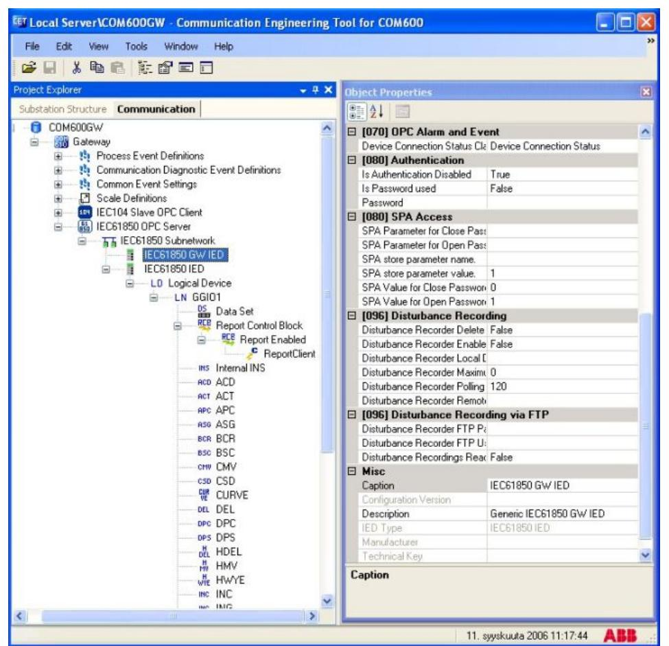
Figure 3.2.1-1 Example view of the Communication Engineering Tool
