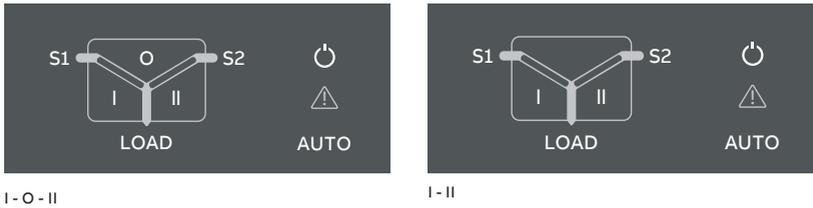
Fig. 9 On left: LEDs in ZTSD, delayed transition, I - O - II. On right: LEDs in ZTS, open transition I - II.
