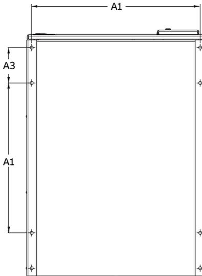
Fig. 21 Automatic transfer switches, Mounting hole dimensions, refer to Table 15
