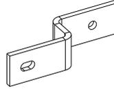
USE BONDING BAR SUPPLIED WITH THE EQUIPMENT
