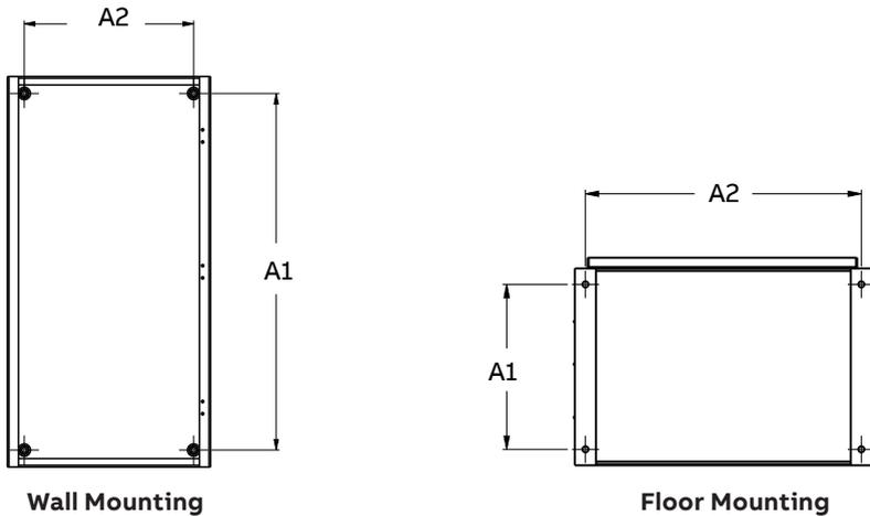
Fig. 20 Automatic transfer switches, Mounting hole dimensions, refer to Table 13 and 14
