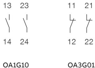
Fig. 22 Labels for contact numbering
