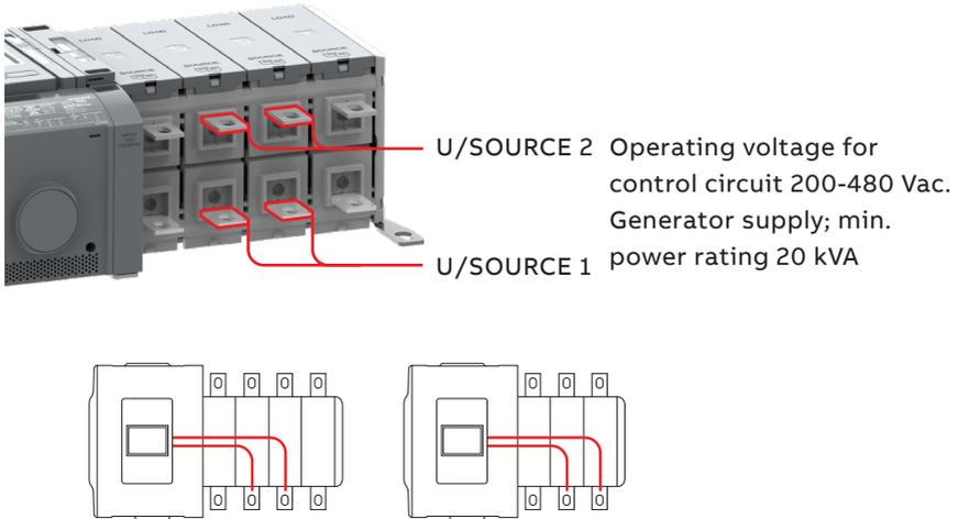
Fig. 12 Power supply for control and power switching circuits
