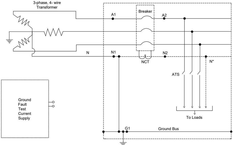
Fig. 6 Main circuit breaker with integral ground fault protection - 3-Phase, 4-wire
