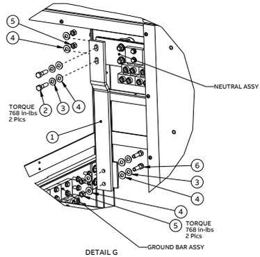
STEP-2: ASSEMBLE BONDING BUSBAR
