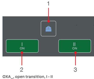
Fig. 11 Keypad in Level 4 HMI with touch screen
