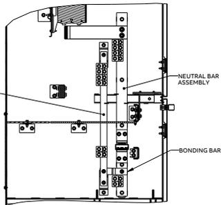
VIEW SHOWING BONDING BAR CONNECTION
