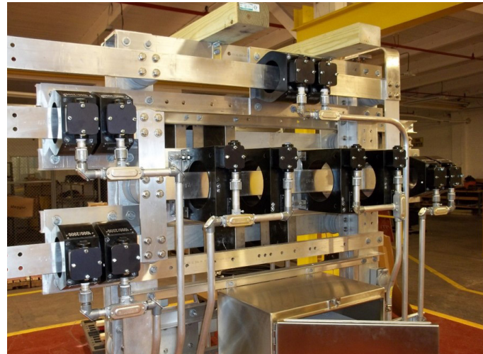
Custom Buss Fabrication and CT Racks
