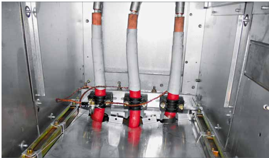
7 40 kA arc effects with AE intervention
