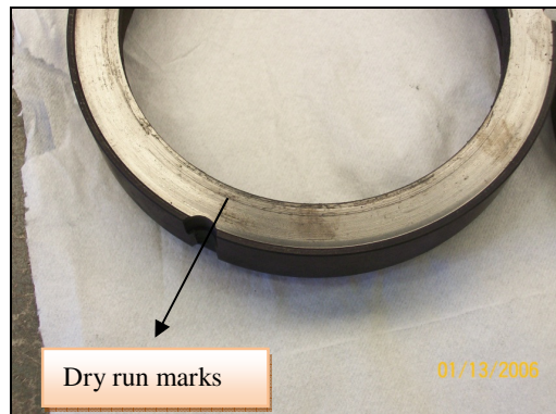
Figure-2. Seal face with lack of lubrication marks
