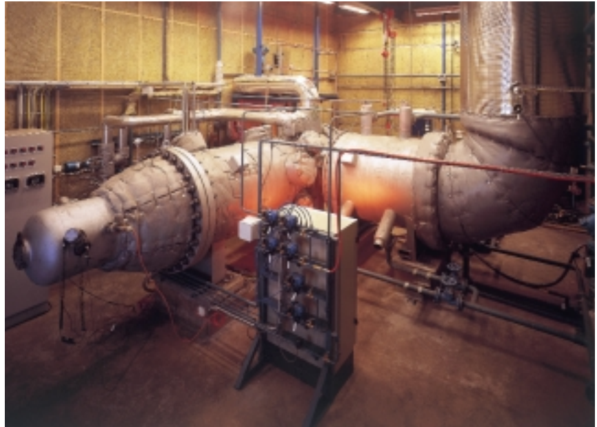
Hot test rig used to verify the advanced turbine cooling technology
