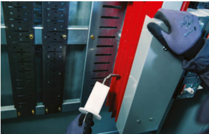
— IP20 compliance for "finger-safe" vertical bus stack assembly as determined by testing with calibrated probe.
