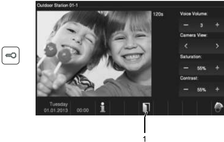
Fig. 8 Opening the door
